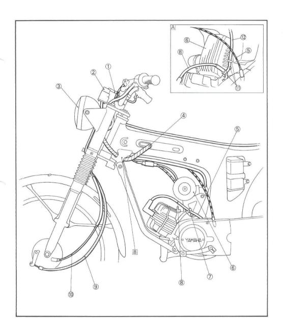
A Fit wire cylinder on to frame tab.
