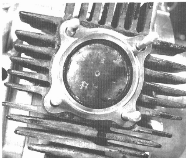
39.7 Use a new cylinder head gasket
