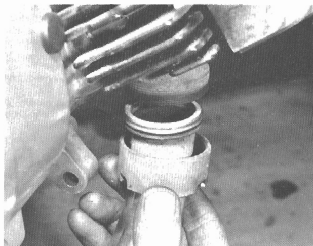
40.2 Use new ring gasket at exhaust pipe joint
