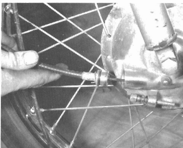
2.4b ... pull cable from housing to disconnect drive
