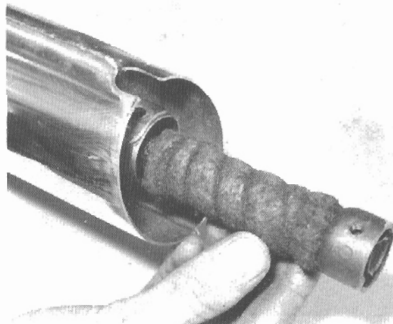
10.7 Avoid burning felt if blowlamp is used to burn out carbon
