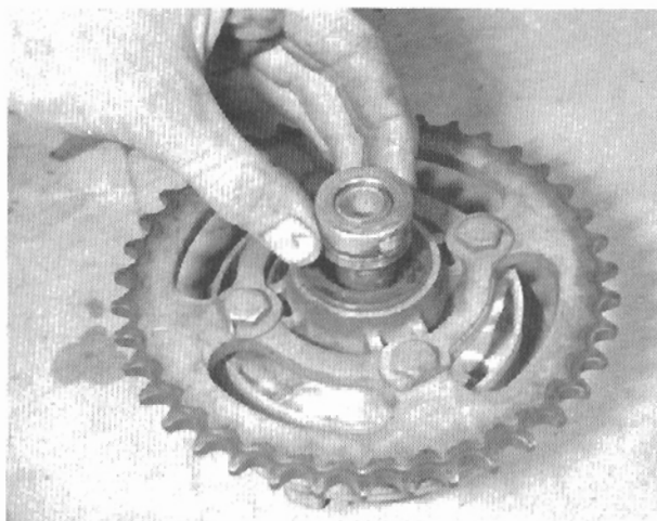
12.1a Rear wheel sprocket bolts to shock absorber plate ...
