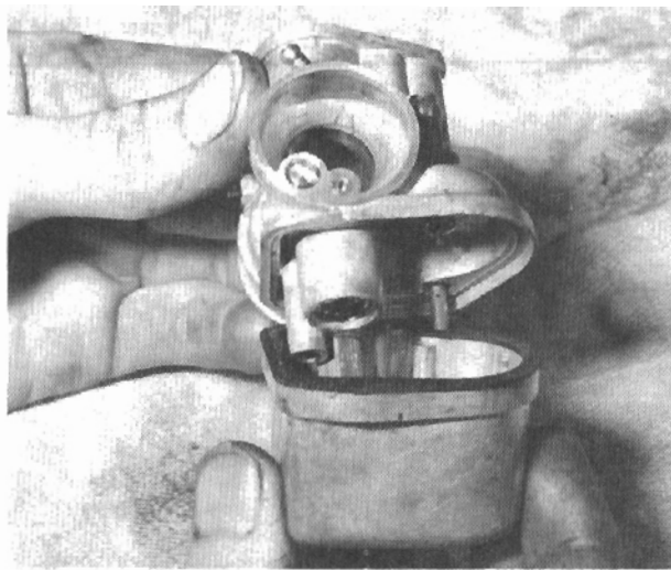
7.2 Release screw at base of carburettor to free float chamber
