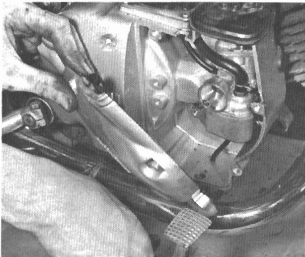
5.13 Remove right-hand cover for access to carburettor
