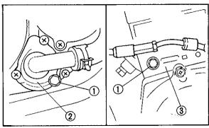
1. Drain bolts 2. Hosing cover 3. Cylinder
