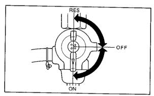
OFF: With the lever in this position, fuel will not flow. Always return the lever to this position when the engine is not running.
