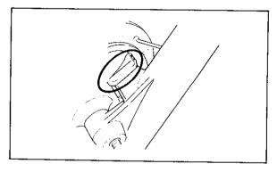
3. Make sure the axle nut is properly torqued, and a new cotter pin is installed.
