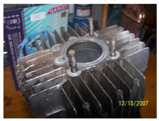
Slide the head off of the studs, leaving the cylinder exposed. It might take just a little wiggling but as long as it's not seized, it should slide right off.
