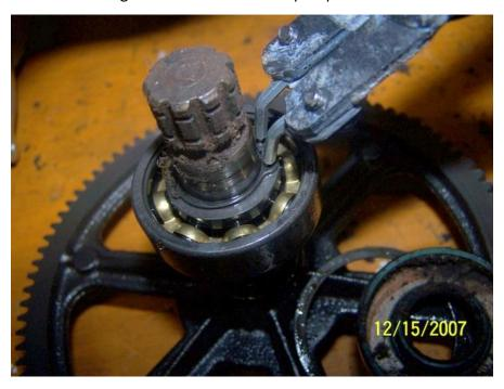
To remove this bearing, I used a three jaw puller as pictured.
