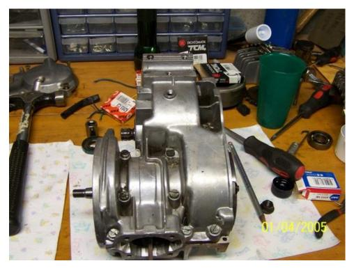
Here is the engine with both halves together.
