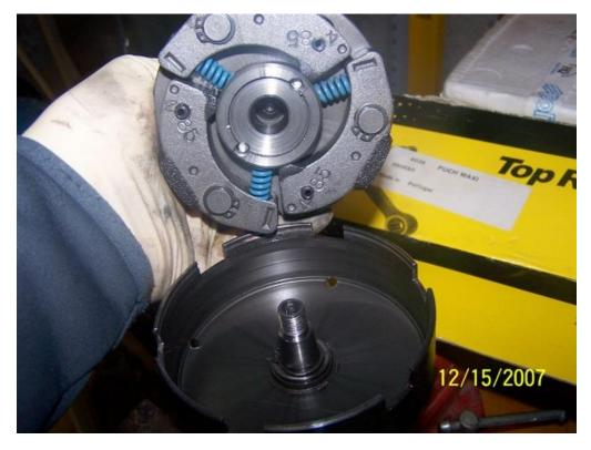
Remove the circlip in the clutch drum. There is a washer underneath it that can slide off too.
