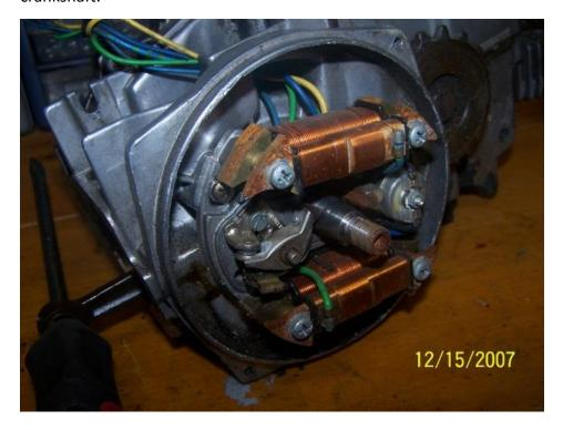
Remove the three screws that hold the stator plate in place.
