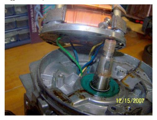
There is a little rubber grommet that the wires go through. This is so that water does not get in to your flywheel area. Slide this off the ends of the wires so that you can pull wires through that hole in the engine case. You should be able to fully remove the stator plate from the engine now.
