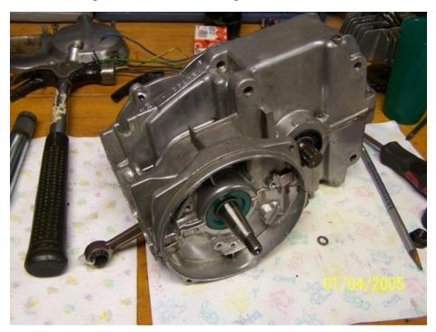
Pull the wires from the stator plate through the hole on top of the engine.
