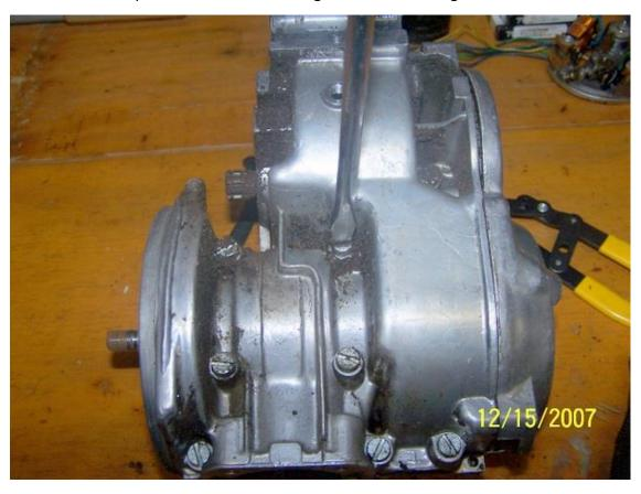
Then I removed the clutch cover by removing the four screws there.
