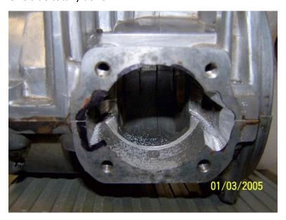
Both sides done. At this point, you can take a finer griding device and smooth it out a bit as this surface is a bit rough. You can even follow it up with some polishing if you'd like. I don't go very deep in to the cases. Just enough to smooth out the transition a bit.
