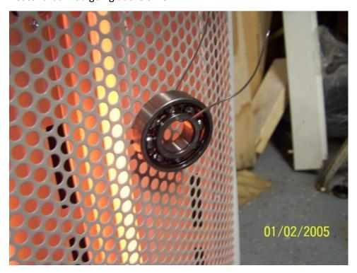
Drop the bearing on to the shaft. It is to rest against the circlip that is closest to the big gear on the shaft. If it doesn't drop right down then take a Puch seat post and pound it down. You want to pound on the inner race of the bearing and not the outer race.
