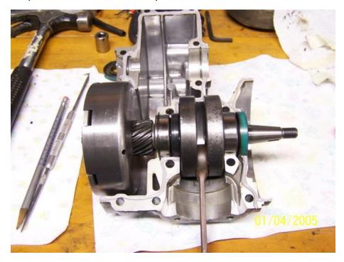
Drop in the drive gear assembly. Put some oil on the part of the case where the non-bearing end of the drive shaft sits. This will help lube it up a bit.
