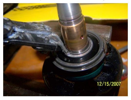
This bearing is a bit trickier since you can't get a three jaw puller on it. Since you are replacing it, it is OK to mangle it. You can try to heat it up and hope to loosen it up or you can try the two screwdriver method to pop it up a bit. Sometimes this will raise it up enough to use a puller.
