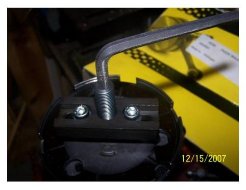
After you break the clutch loose, remove it. This is a three shoe clutch. In a stock Puch engine, you will more than likely find a two shoe clutch so yours may look a little different.
