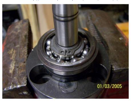
Place the larger washer on top of the circlip.
