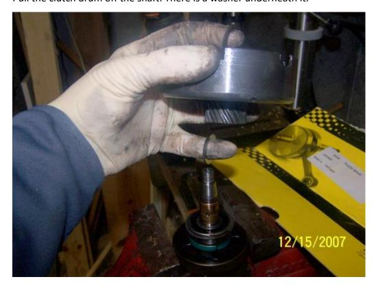
Remove the other circlip on the shaft. Also, remove the bushing.
