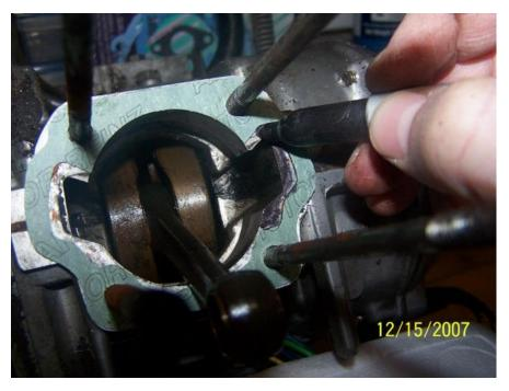
Here is what it looks like with the base gasket removed. Anything marked in black needs to be removed so that air flow can be improved with the performance kit. You can install a kit without case matching but if you really want to see some improvements do the case match.
