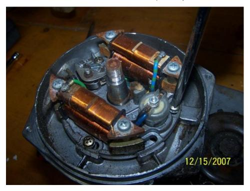
Wiggle it a bit and pull it off. The wires will still be attached.
