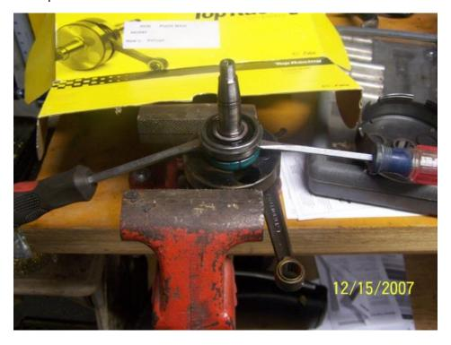
A ball joint fork (for cars) works well for this. Both methods will destroy your seal though so plan to replace them. In the picture I didn't have the upper circular part in the vice. Make sure you do that so that the forces on your crank don't deform it.
