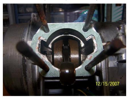
Then I marked where the ports need to be opened with a Sharpie so that I know what material to remove from the engine case.
