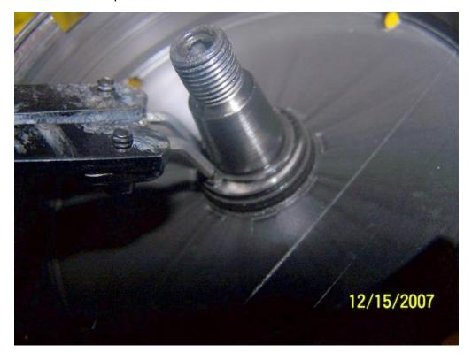
Pull the clutch drum off the shaft. There is a washer underneath it.
