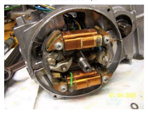
Install the flywheel (don't forget to put that little semi-circle (woodruff key) piece back in before you install it!) and you're ready to install your piston, cylinder and head and you'll be back in business. Anytime you do a rebuild, it's a good idea to go a little heavier with the gas/oil mix to help break it in. Vary your speed and don't go full out right away. Let things settle in a bit.
