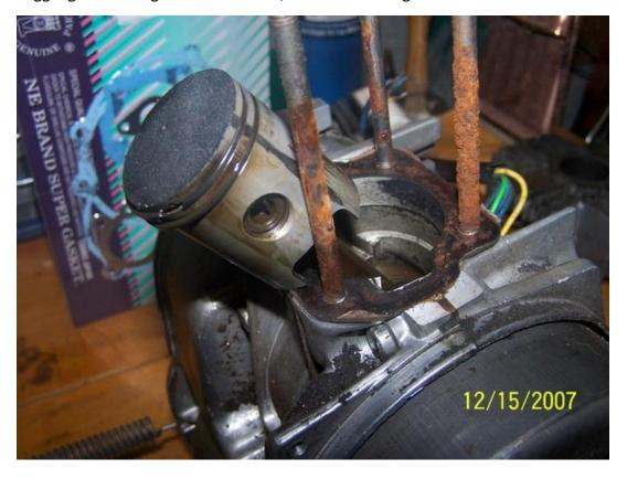
Remove the little retaining clip that is holding the piston on the wrist pin. Use a small pair of pliers for this. Do it on both sides of the piston.
