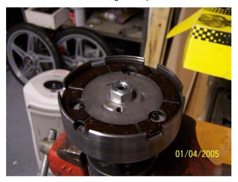
Put the starting plate back and reinstall the retaining ring.
