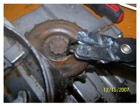
Once that circlip is removed you should be able to pull the sprocket off of the end of the shaft. There will be another circlip behind it. Remove it.
