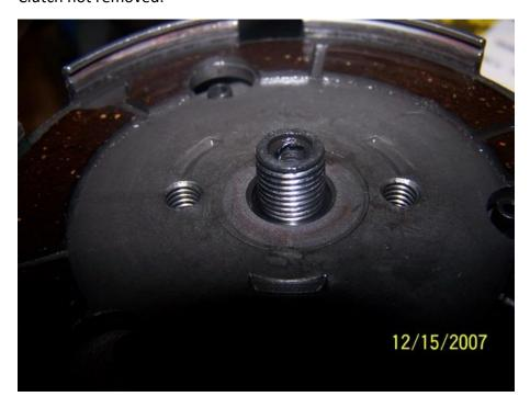
Use a clutch puller to remove the clutch. This is a purchased specialty tool but you can make one also.
