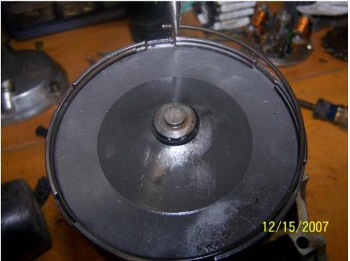
Remove the clutch starting plate.
