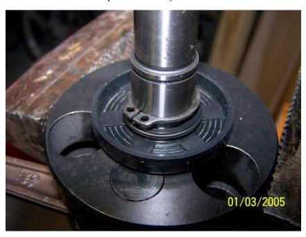
Next, install the bearing with the retaining ring towards the outside of the shaft. Pound it down until it makes contact with the circlip. Install the other circlip on top. POSSIBLE CORRECTION: OIL SEAL PLACEMENT
