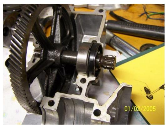
Grab the crankshaft and let's work on that one now. Remove the large retaining ring from the clutch.
