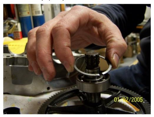
Lube up the seal and install it with the lips facing out.
