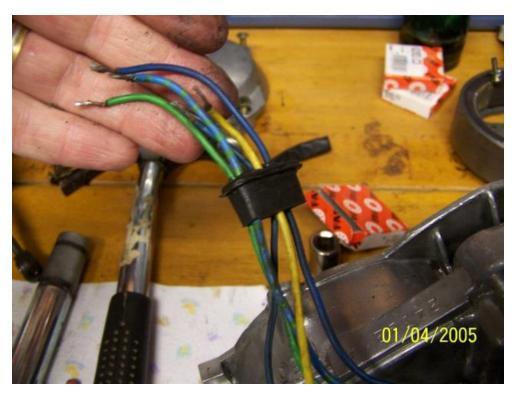
Screw the stator plate back on with the three screws. You can read how to set the timing from other sources once it is back on the moped.
