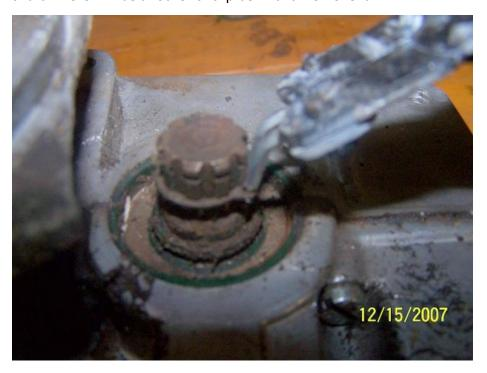
I then loosened up all of the screws holding the two halves together. There are 13 of them.
