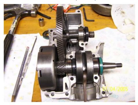
Make sure the seals are where you need them to be and pop the other case half on and start screwing. Work in a criss-cross fashion when tightening down the screws.
