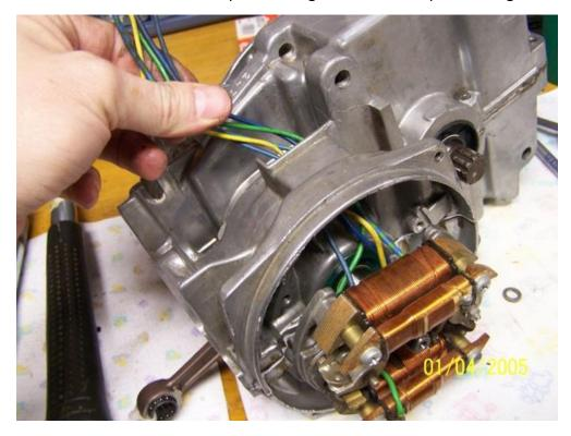
Feed the wires through that rubber grommet and slide it down the wires until it is firmly in the hole.
