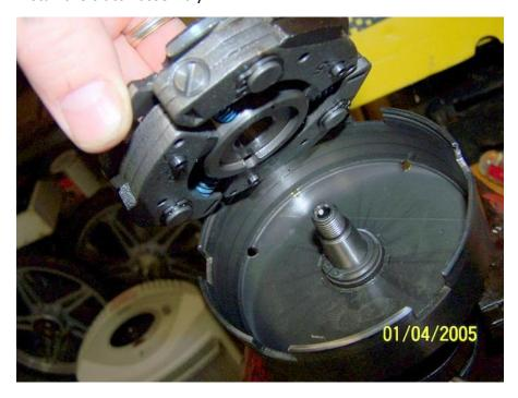
Put on the washer and nut and tighten it up.
