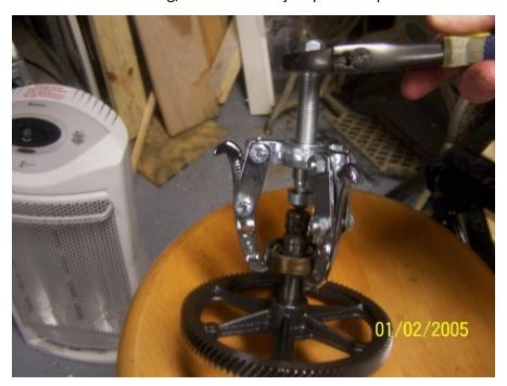
To install a new bearing heat up the new bearing in an oven at 300 degrees for ten minutes or so. This will cause it to expand, making it easier to install. I hung mine in front of my heater that I had going at the time.
