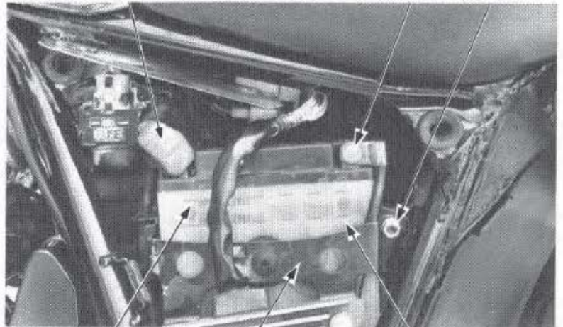
(4) UPPER LEVEL (5) BATTERY HOLDER (6) LOWER LEVEL
