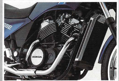
Compact, 52° V-twin configuration.
