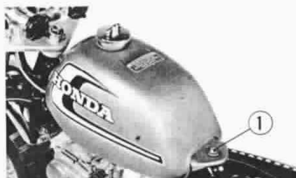
① Setting 6 mm bolt Fig. 49
