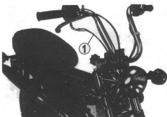
Fig. K4-5 ① Throttle cable
