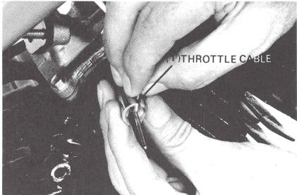
Slide the throttle valve into the carburetor-body.
