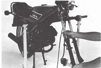
Tighten the right and left fork pinch bolts to the specified torque.
