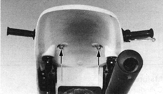
2. Remove the three bolts from the side cover assembly and two bands.
