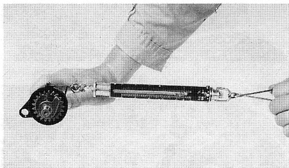
2. Check the clip for damage and wear, and determine whether or not, it should be replaced.
