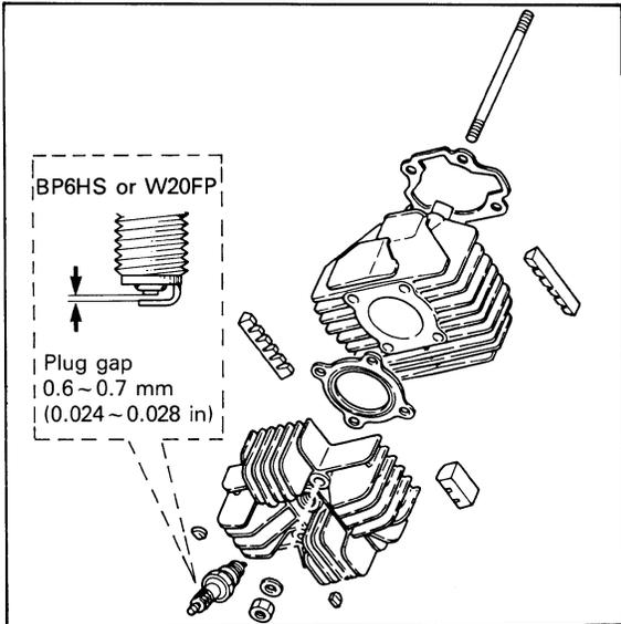
3. With the piston at top dead center, raise the cylinder until the cylinder skirts clear crankcase. Stuff a clean shop rag into crankcase cavity, around rod, to prevent dirt and other foreign particles from entering. Remove cylinder.
