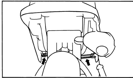
2. Turn the fuel cock to "OFF" and disconnect the fuel pipe.
