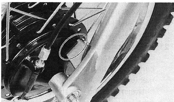
2. Tighten the axle nut.
