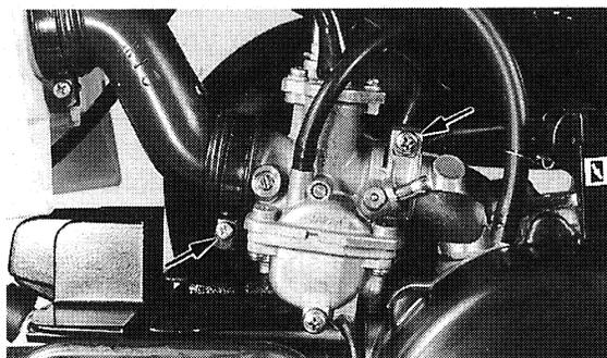
4. Rotate the carburetor, remove the mixing chamber top, and carburetor assembly.
