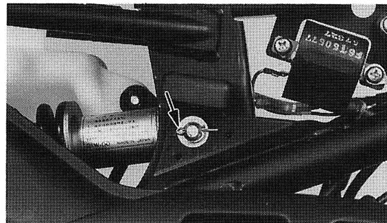
6. Remove the cotter pin and remove the pin from the swingarm.
