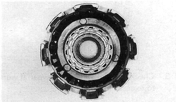
7. Measure the gap between the friction plate and pressure plate with a thickness gauge.
