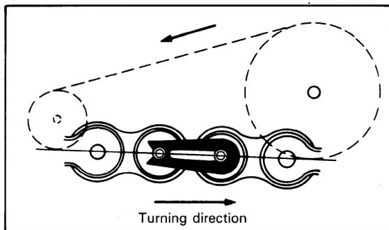
2. Be sure to adjust the chain slack. (Refer to "Drive chain slack adjustment".)
