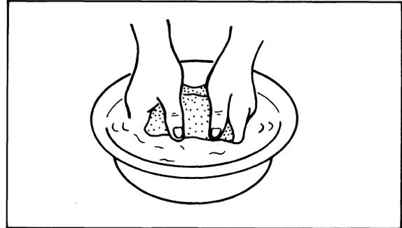
4. Squeeze the solvent from the filter element.
