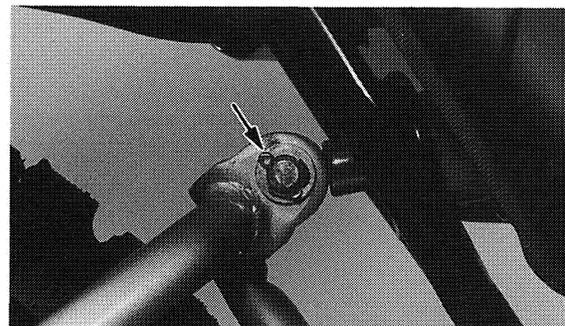
7. Remove the rear shock absorber from the machine. (To remove, pull the rear shock backward while lifting up the frame.)
