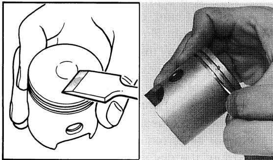
3. Using 400 ~ 600 grit wet sandpaper, lightly sand score marks and lacquer deposits from sides of piston. Sand in a crisscross pattern. Do not sand excessively.
