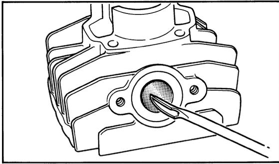
2. Check cylinder bore. Using a cylinder hone, remove any scoring. Hone lightly, using smooth stones. Hone no more than required to avoid excess piston clearance.
