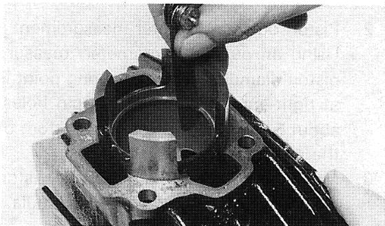
3. With rings installed in grooves, insert feeler gauge between ring and groove. If beyond tolerance, replace ring and/or piston as required.
