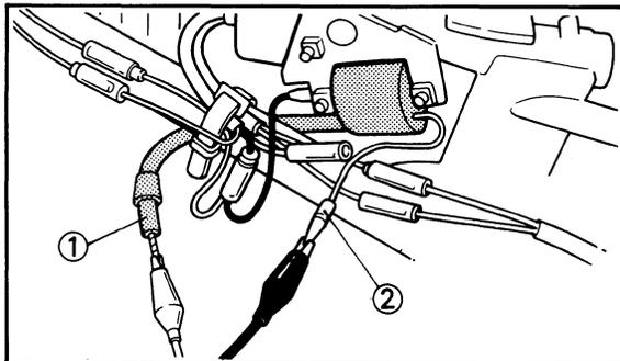
Tester (+) lead → Spark plug lead ①
