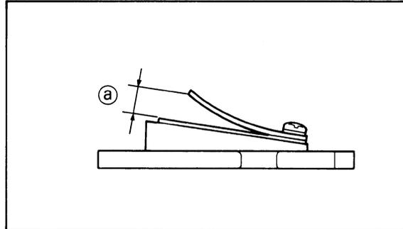
4. Check reed valve for bending. If beyond tolerance, replace reed valve.
