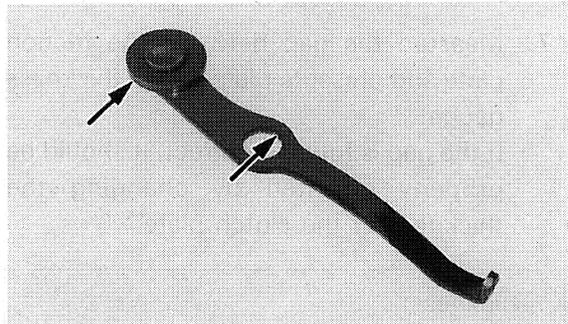
4. After installation of the shift shaft, check the clearances A and A' (between the prongs of shift lever 1 and shift drum pins) are equal.
