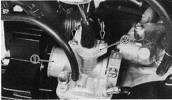
1. Carburetor                      2. Mixing chamber top
