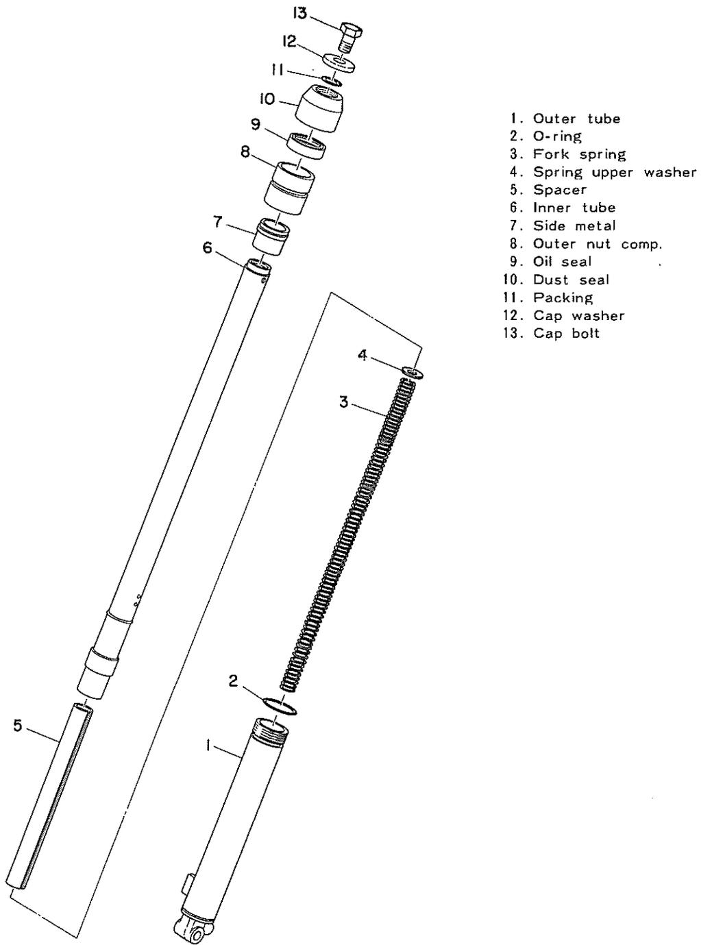
Fig. 5-5-7 Front Exploded View
