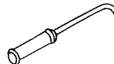
Insert the bent end of the special tool into the hole located in the center of the bearing space.
