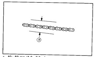
a  $40\sim50 \text{ mm} (1.6\sim2.0 \text{ in})$  EAI41400
