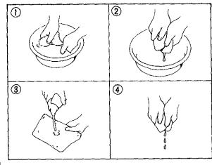
4. Apply recommended oil to the entire surface of the filter and squeeze out the excess oil The element should be wet but not dripping.
