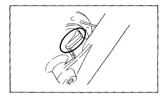
3 Make sure the axle nut is properly torqued, and a new cotter pin is installed.
