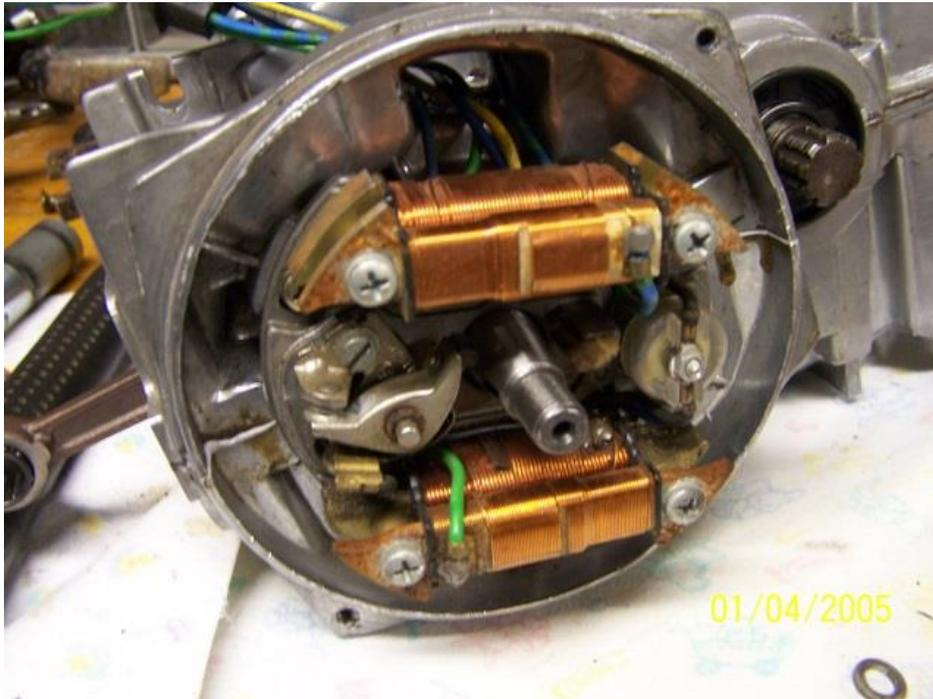
Install the flywheel (don't forget to put that little semi-circle (woodruff key) piece back in before you install it!) and you're ready to install your piston, cylinder and head and you'll be back in business. Anytime you do a rebuild, it's a good idea to go a little heavier with the gas/oil mix to help break it in. Vary your speed and don't go full out right away. Let things settle in a bit.
