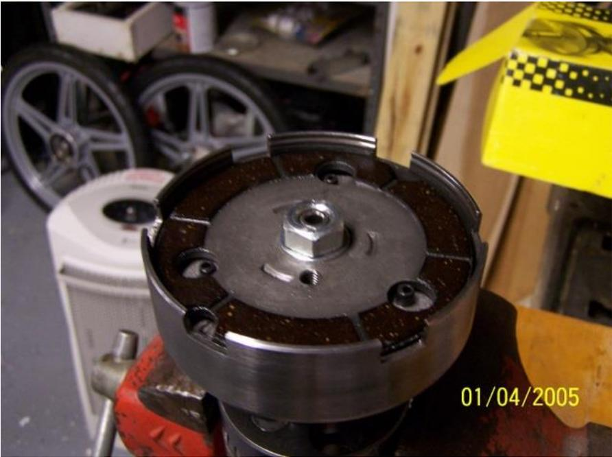
Put the starting plate back and reinstall the retaining ring.
