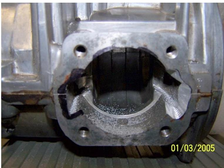
Both sides done. At this point, you can take a finer grinding device and smooth it out a bit as this surface is a bit rough. You can even follow it up with some polishing if you'd like. I don't go very deep in to the cases. Just enough to smooth out the transition a bit.
