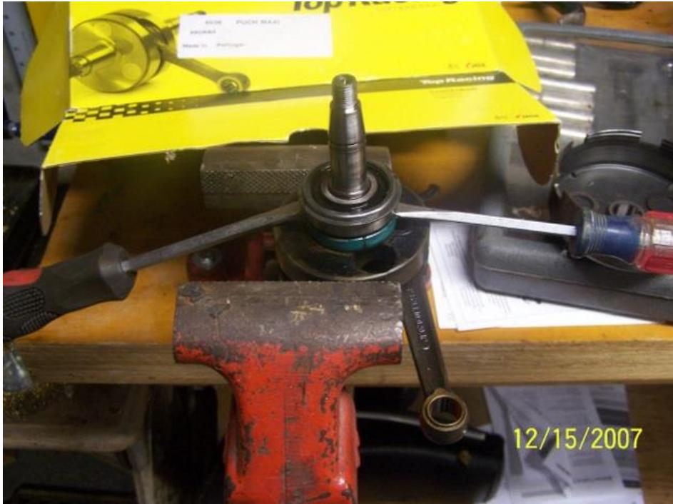
A ball joint fork (for cars) works well for this. Both methods will destroy your seal though so plan to replace them. In the picture I didn't have the upper circular part in the vice. Make sure you do that so that the forces on your crank don't deform it.
