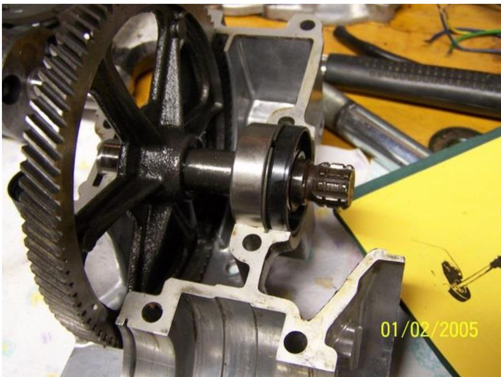
Grab the crankshaft and let's work on that one now. Remove the large retaining ring from the clutch.
