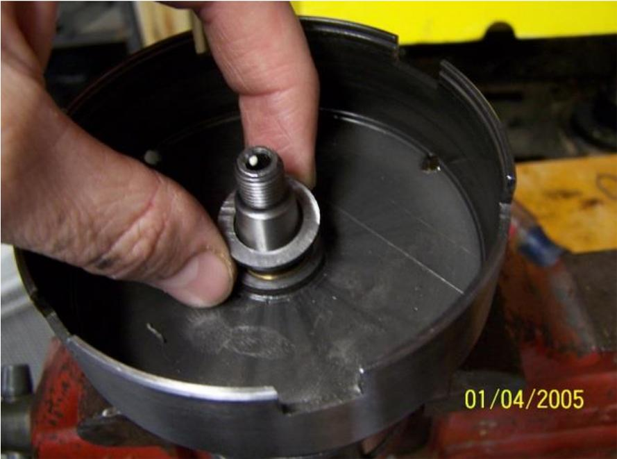
Install the circlip.
