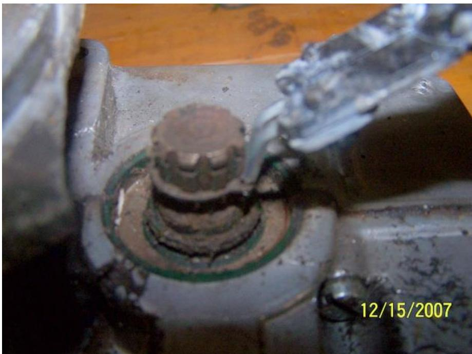
I then loosened up all of the screws holding the two halves together. There are 13 of them.
