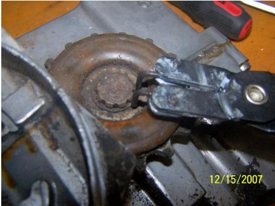
Once that circlip is removed you should be able to pull the sprocket off of the end of the shaft. There will be another circlip behind it. Remove it.
