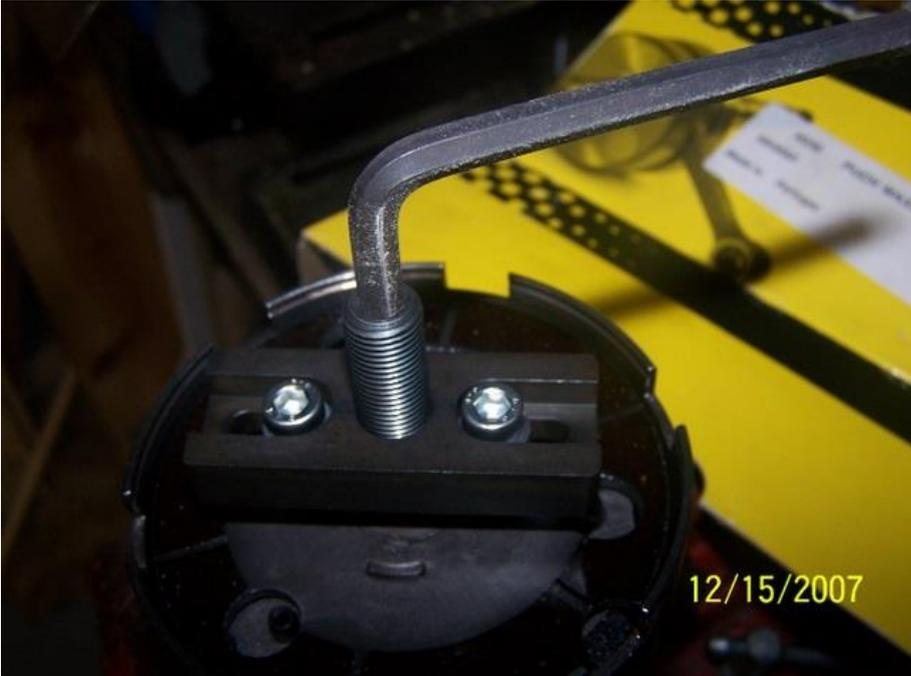
After you break the clutch loose, remove it. This is a three shoe clutch. In a stock Puch engine, you will more than likely find a two shoe clutch so yours may look a little different.
