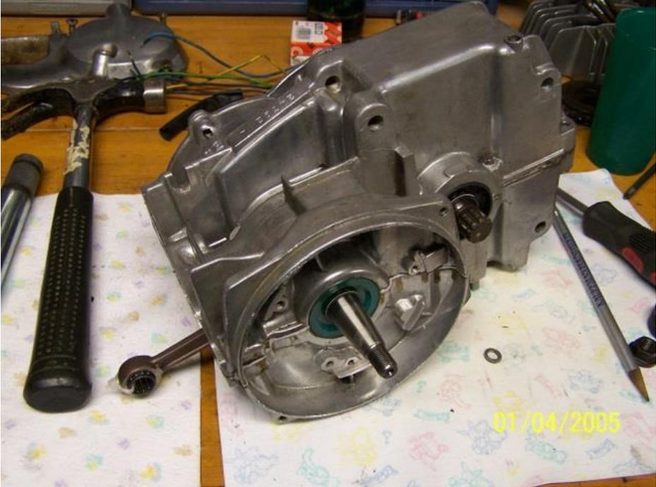
Pull the wires from the stator plate through the hole on top of the engine.
