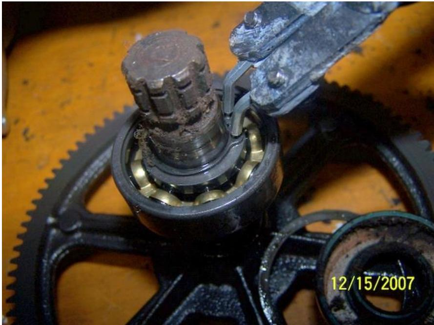
To remove this bearing, I used a three jaw puller as pictured.
