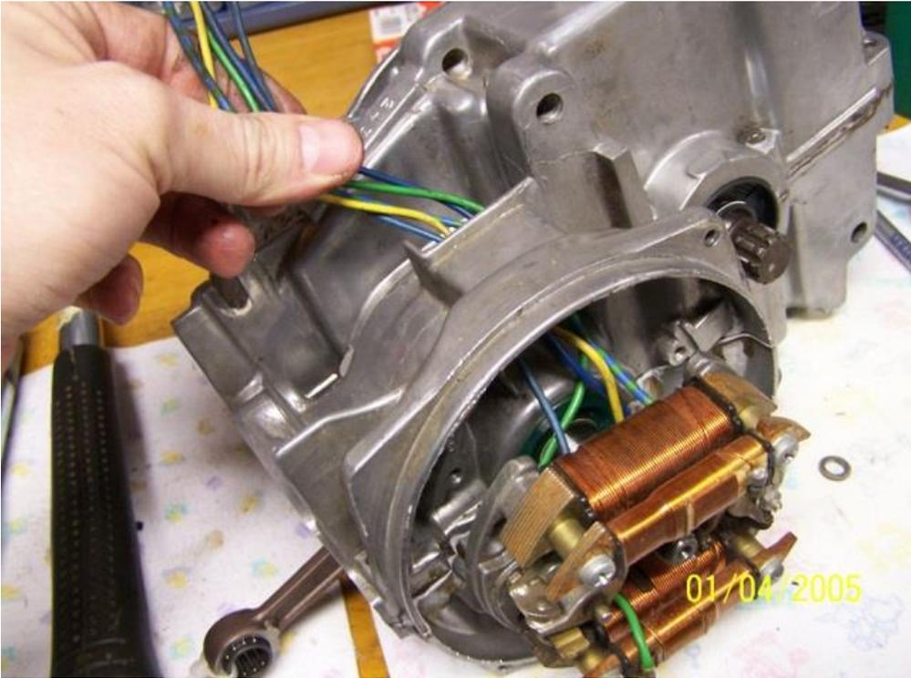
Feed the wires through that rubber grommet and slide it down the wires until it is firmly in the hole.
