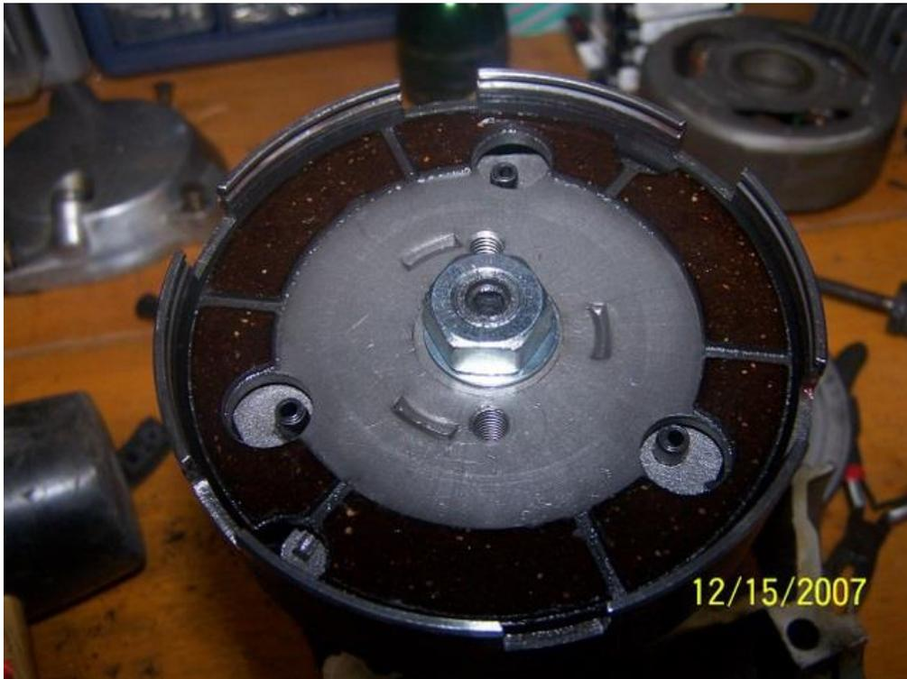
Remove the clutch nut. Removing the clutch would be easier with a piston stop before the engine is off the bike. If you do it goofy like me, then put the circular part of the crank closest to the clutch in a vice and proceed my way. Remember, if you're smart, you'll remove the clutch using a piston stop. Anyway, carry on.
