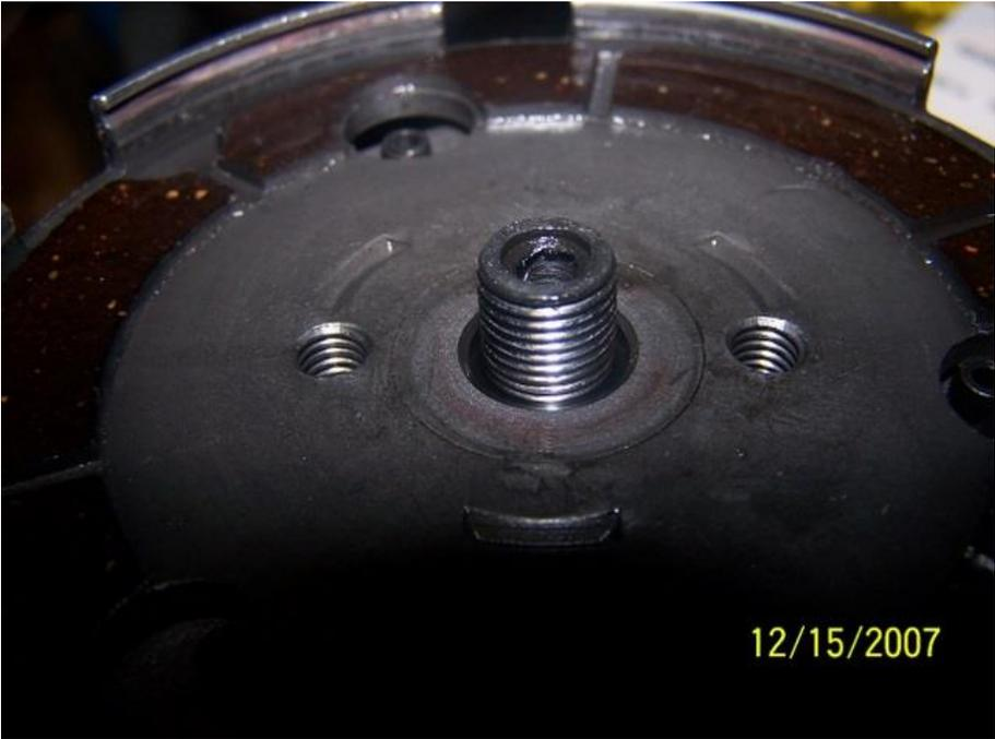
Use a clutch puller to remove the clutch. This is a purchased specialty tool but you can make one also.
