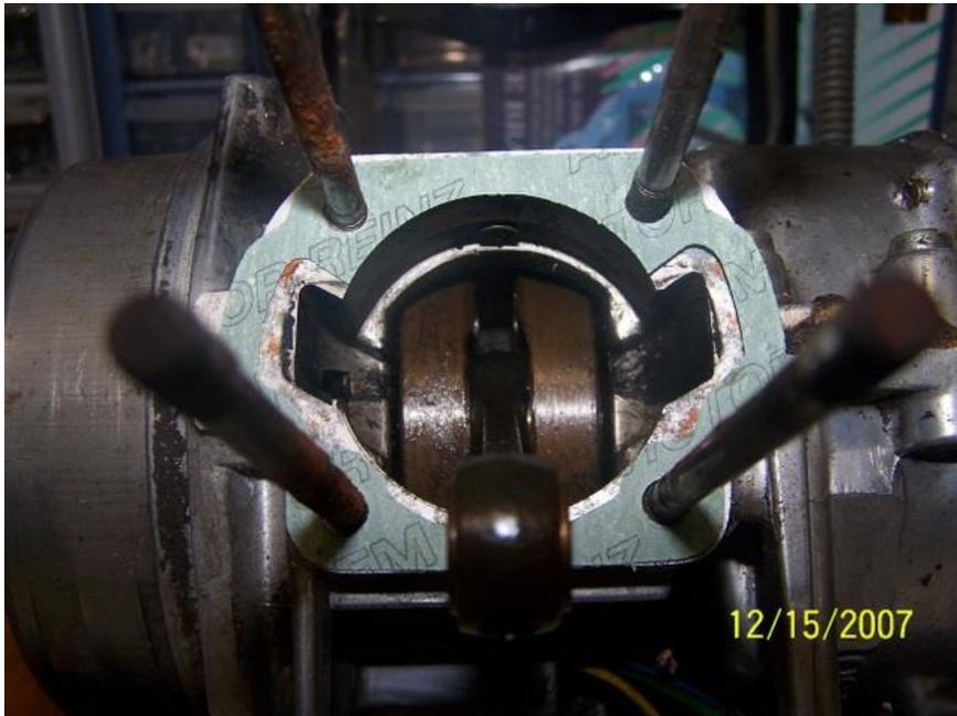
Then I marked where the ports need to be opened with a Sharpie so that I know what material to remove from the engine case.
