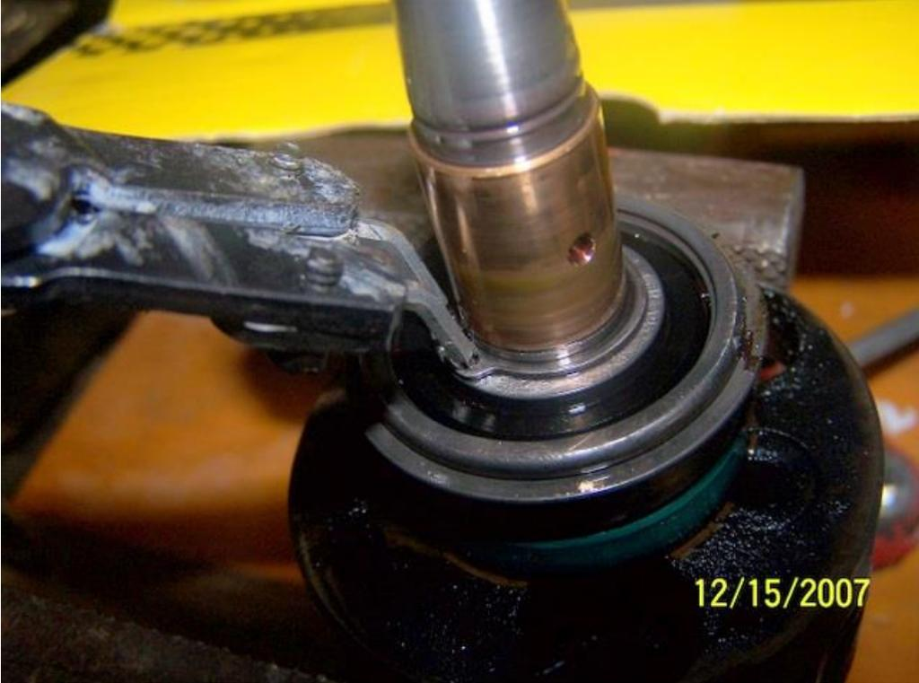
This bearing is a bit trickier since you can't get a three jaw puller on it. Since you are replacing it, it is OK to mangle it. You can try to heat it up and hope to loosen it up or you can try the two screwdriver method to pop it up a bit. Sometimes this will raise it up enough to use a puller.
