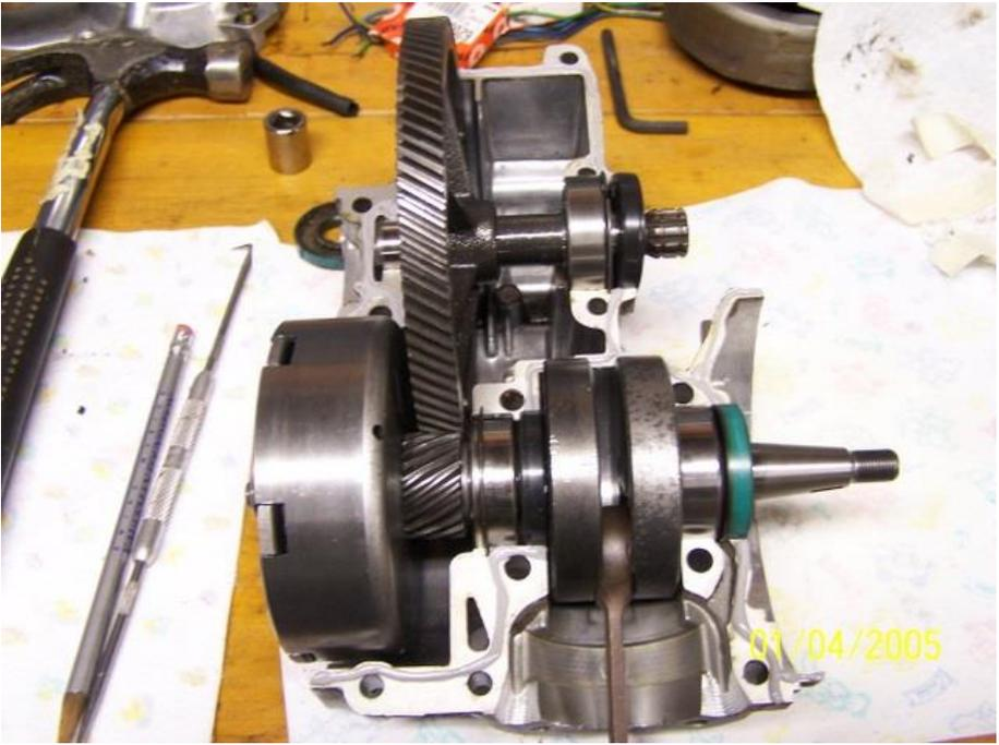
Make sure the seals are where you need them to be and pop the other case half on and start screwing. Work in a criss-cross fashion when tightening down the screws.
