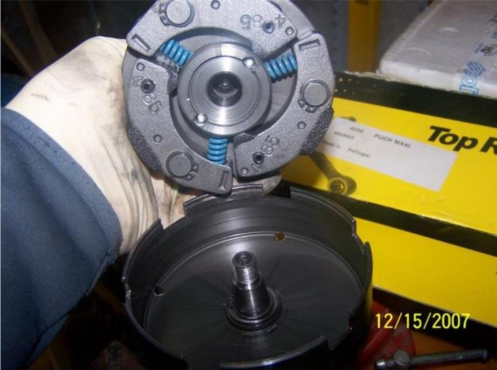
Remove the circlip in the clutch drum. There is a washer underneath it that can slide off too.
