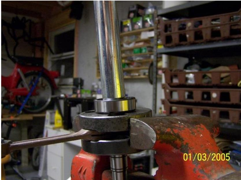
On the clutch side of the shaft, place a seal with the lip facing out and then install a circlip. The circlips locate the bearing on the shaft.
