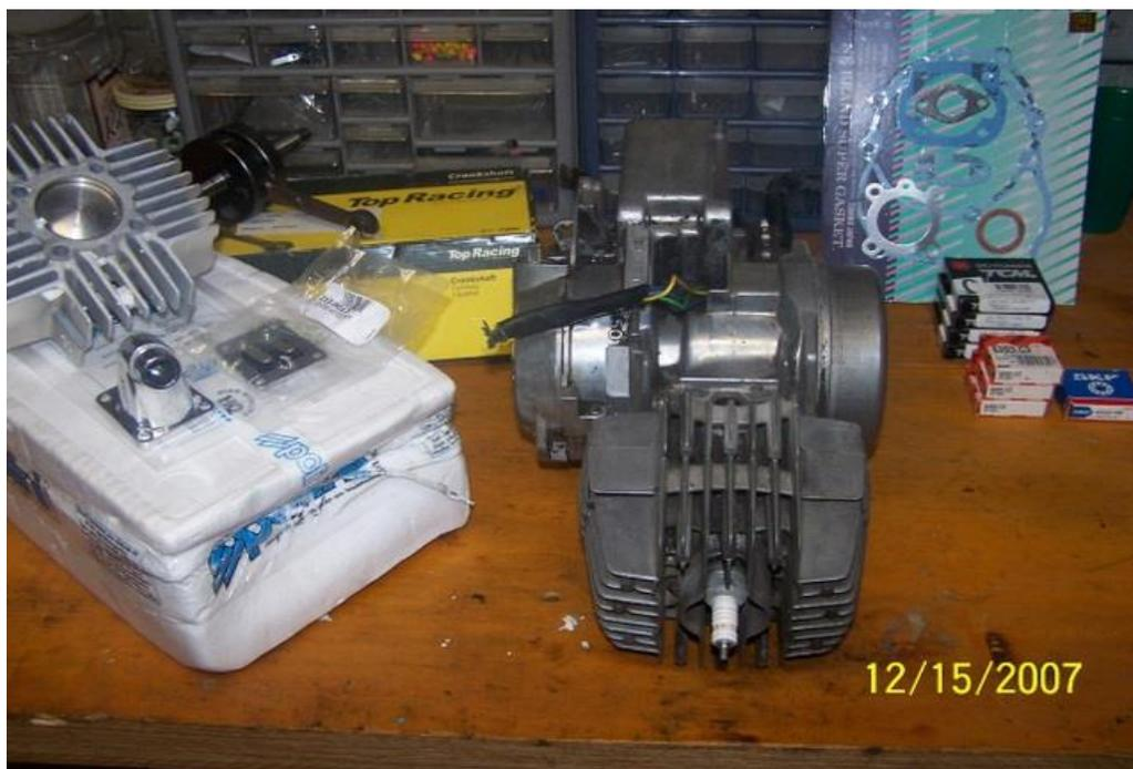
Loosen the four head nuts.
