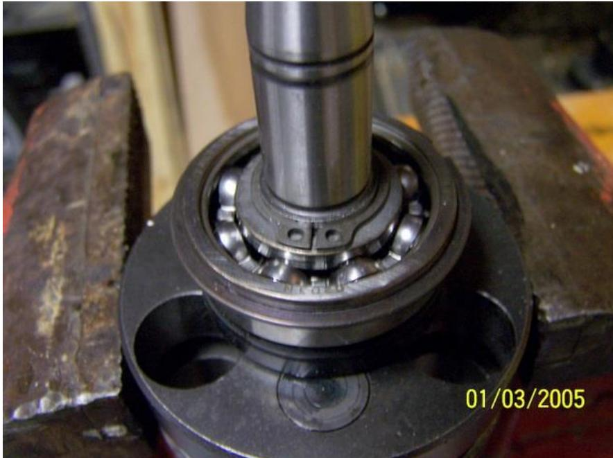
Place the larger washer on top of the circlip.
