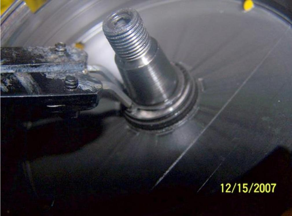
Pull the clutch drum off the shaft. There is a washer underneath it.
