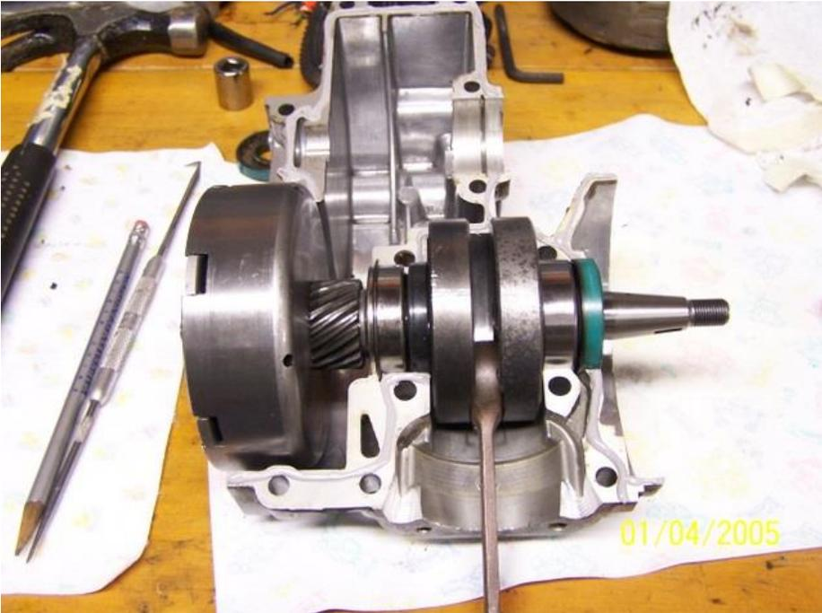
Drop in the drive gear assembly. Put some oil on the part of the case where the non-bearing end of the drive shaft sits. This will help lube it up a bit.
