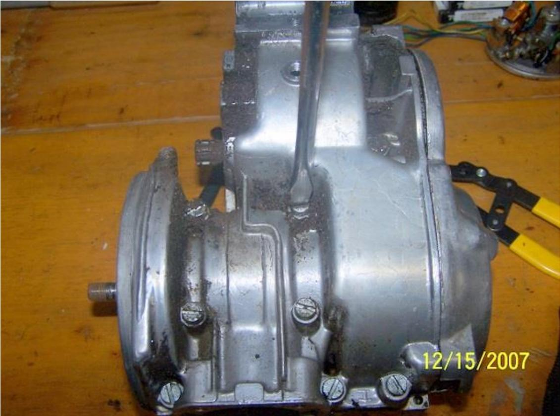
Then I removed the **clutch** cover by removing the four screws there.
