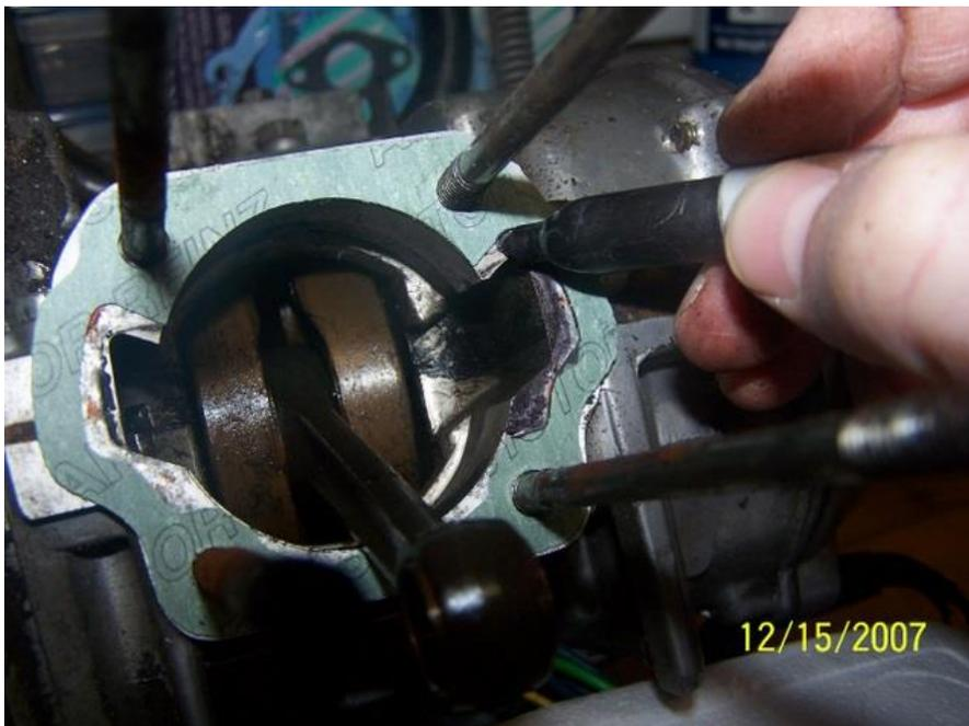
Here is what it looks like with the base gasket removed. Anything marked in black needs to be removed so that air flow can be improved with the performance kit. You can install a kit without case matching but if you really want to see some improvements do the case match.
