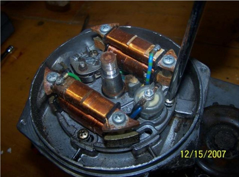
Wiggle it a bit and pull it off. The wires will still be attached.
