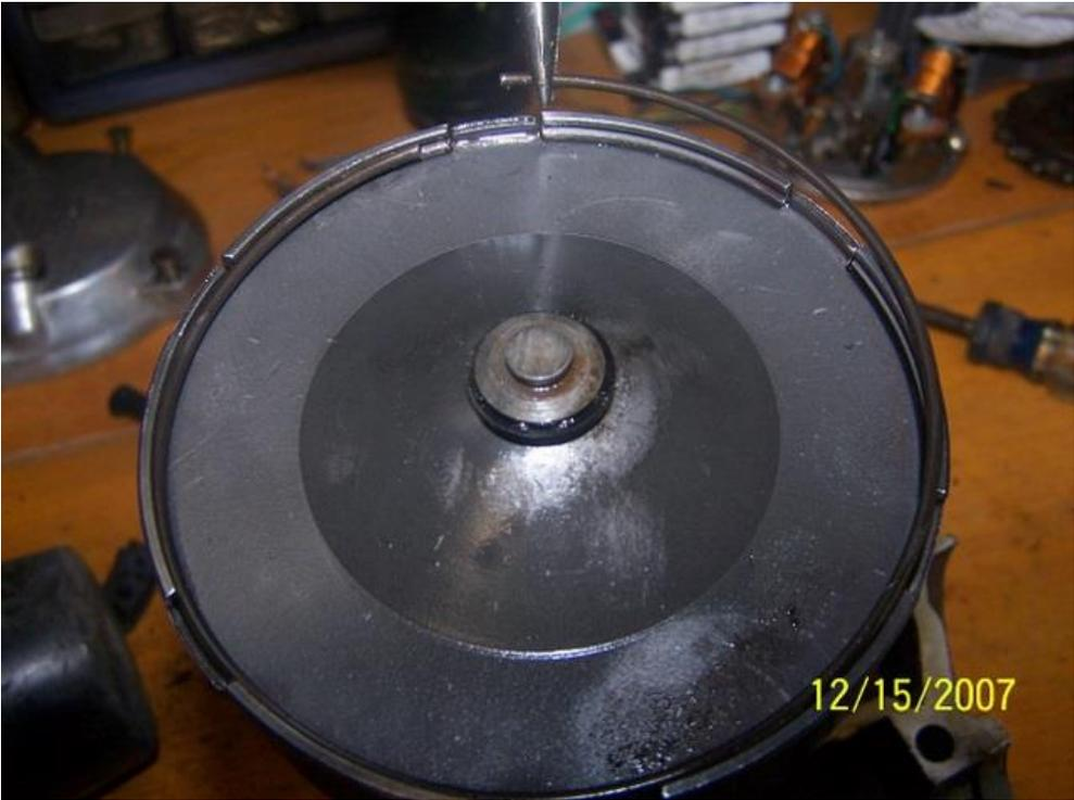
Remove the clutch starting plate.
