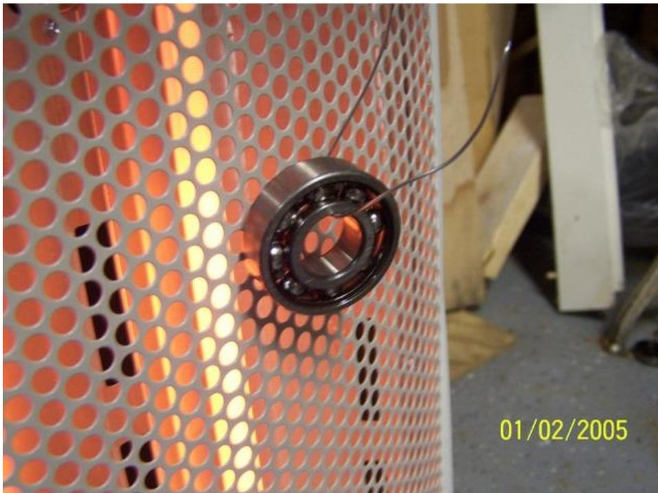
Drop the bearing on to the shaft. It is to rest against the circlip that is closest to the big gear on the shaft. If it doesn't drop right down then take a Puch seat post and pound it down. You want to pound on the inner race of the bearing and not the outer race.
