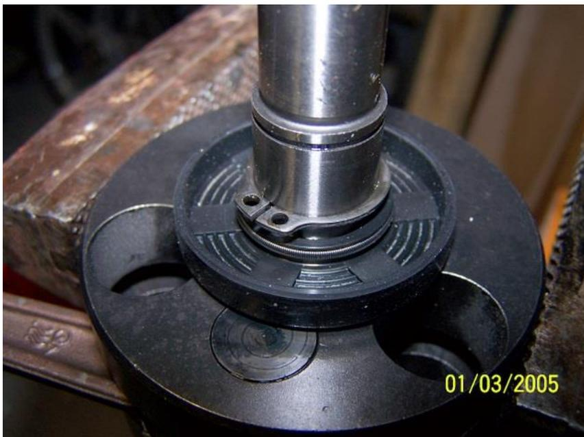
Next, install the bearing with the retaining ring towards the outside of the shaft. Pound it down until it makes contact with the circlip. Install the other circlip on top. POSSIBLE CORRECTION: OIL SEAL PLACEMENT
