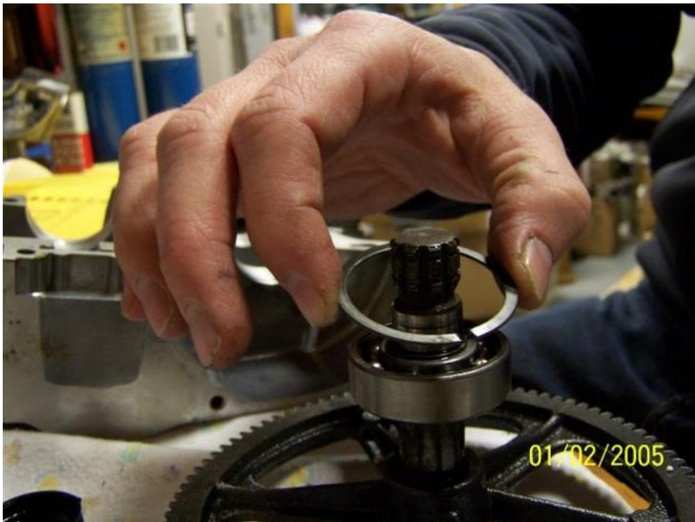
Lube up the seal and install it with the lips facing out.
