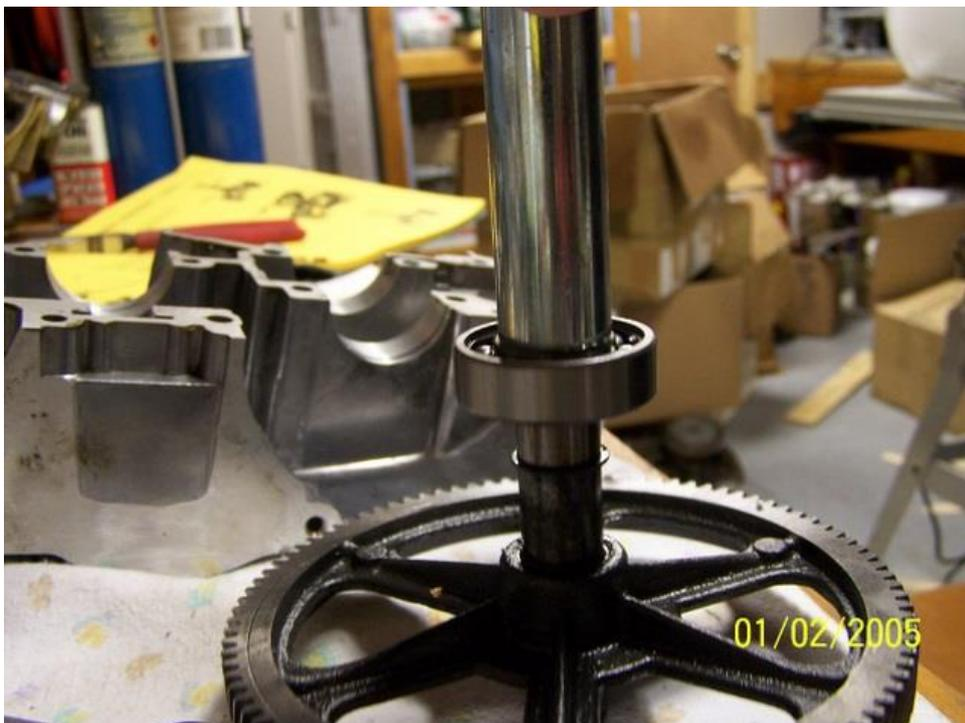
Reinstall the outer circlip.
