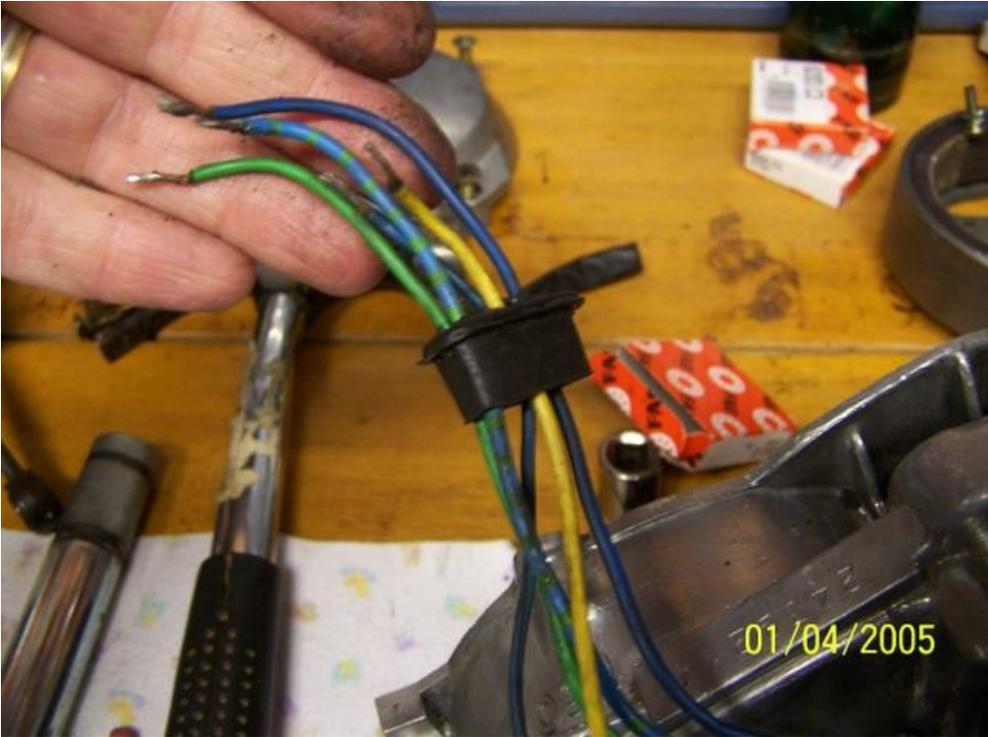
Screw the stator plate back on with the three screws. You can read how to set the timing from other sources once it is back on the moped.
