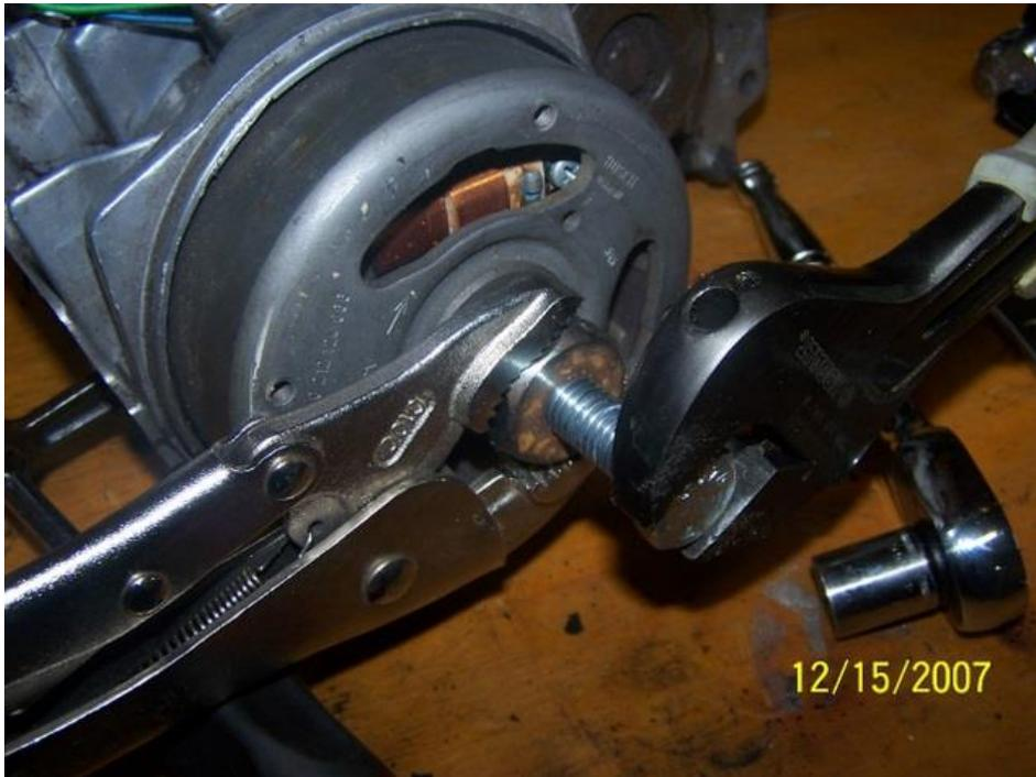
Once you pull off the flywheel make sure that you find the little **woodruff key**. It's the little half-circle piece of metal that makes sure that your flywheel lines up correctly on the crankshaft.
