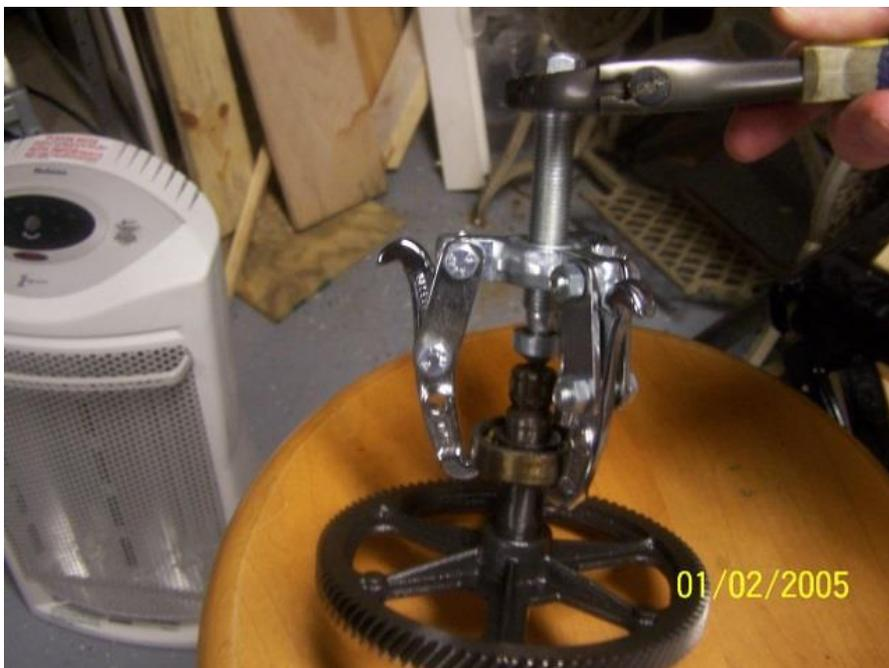
To install a new bearing heat up the new bearing in an oven at 300 degrees for ten minutes or so. This will cause it to expand, making it easier to install. I hung mine in front of my heater that I had going at the time.
