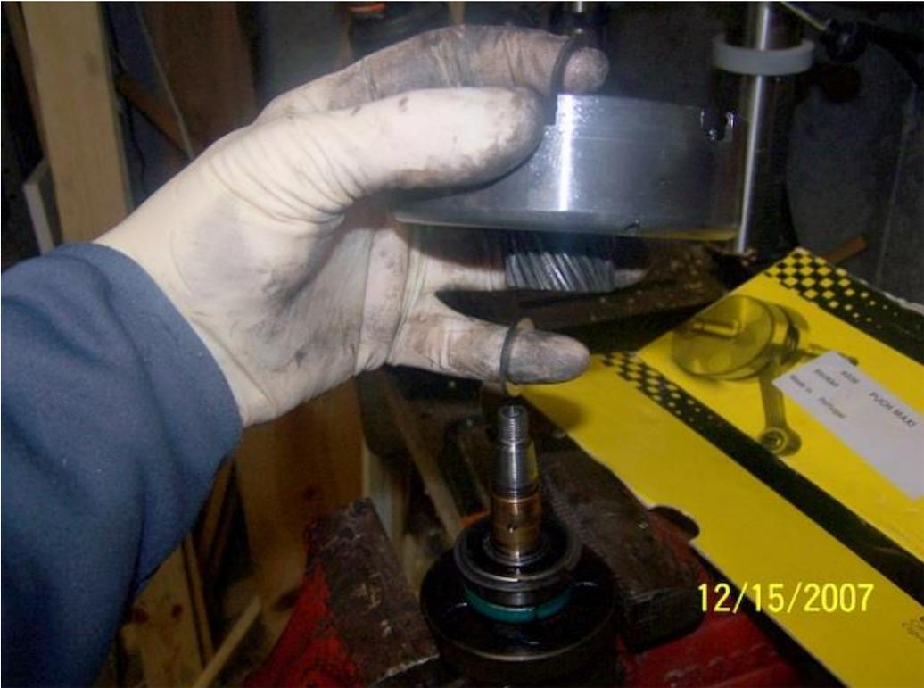
Remove the other circlip on the shaft. Also, remove the bushing.
