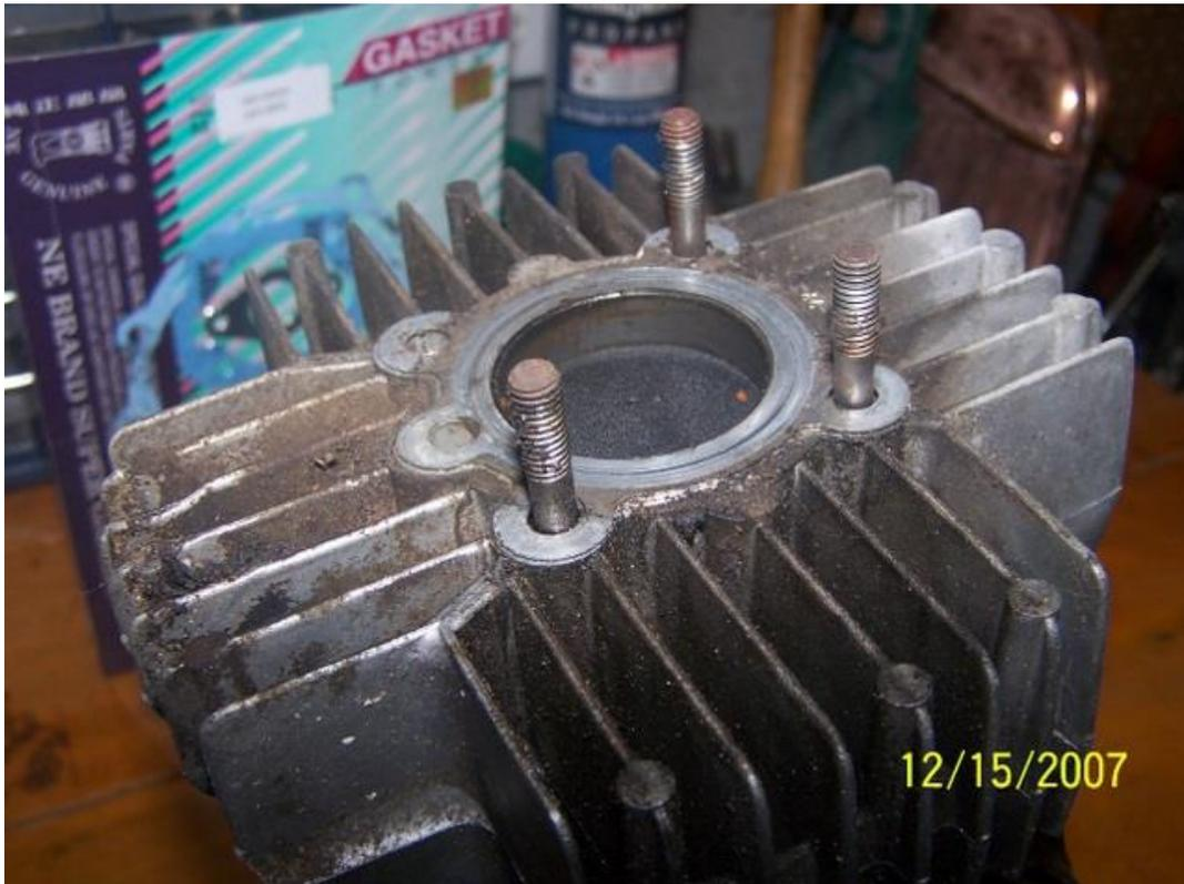
Slide the head off of the studs, leaving the **cylinder** exposed. It might take just a little wiggling but as long as it's not **seized**, it should slide right off.
