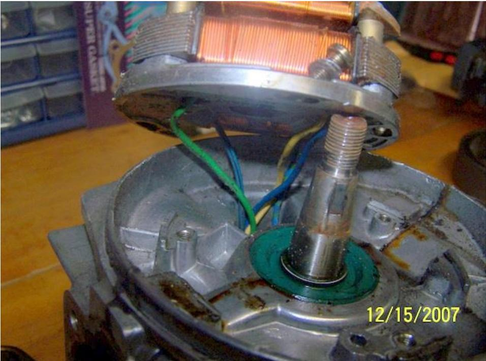
There is a little rubber grommet that the wires go through. This is so that water does not get in to your flywheel area. Slide this off the ends of the wires so that you can pull wires through that hole in the engine case. You should be able to fully remove the stator plate from the engine now.
