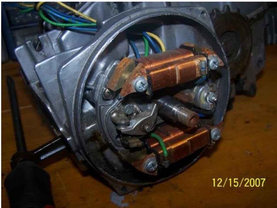
Remove the three screws that hold the stator plate in place.
