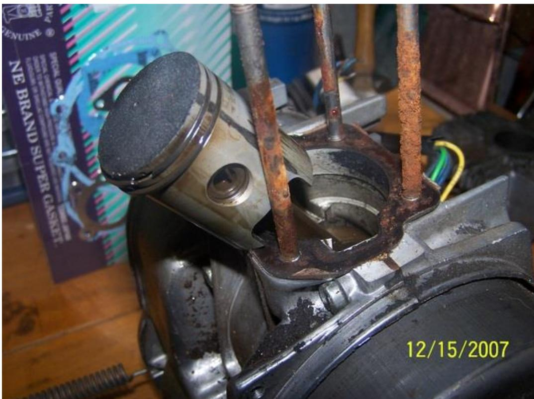
Remove the little retaining clip that is holding the **piston** on the **wrist pin**. Use a small pair of pliers for this. Do it on both sides of the piston.
