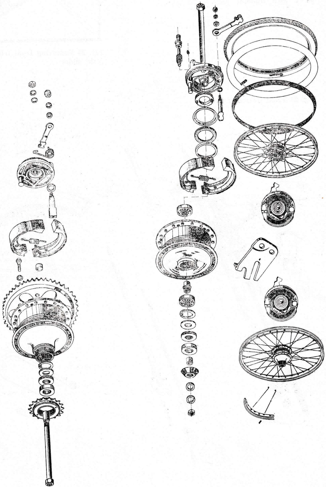
Fig. 26 Exploded view of front and rear wheel.
