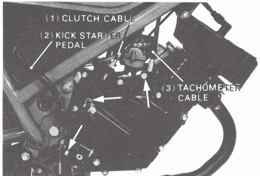
Remove the bolts attaching the right crankcase cover, and remove the right crankcase cover.
