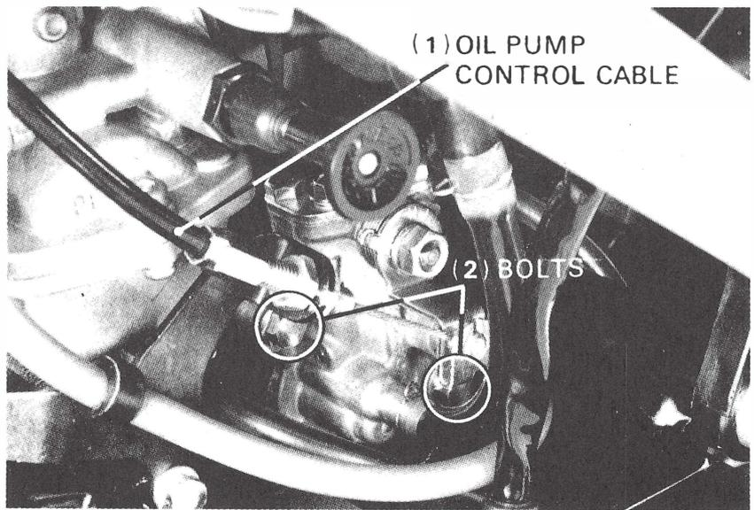
Disconnect the oil pipe from the oil pump, and pinch the end of the oil pipe to prevent oil from flowing out.
