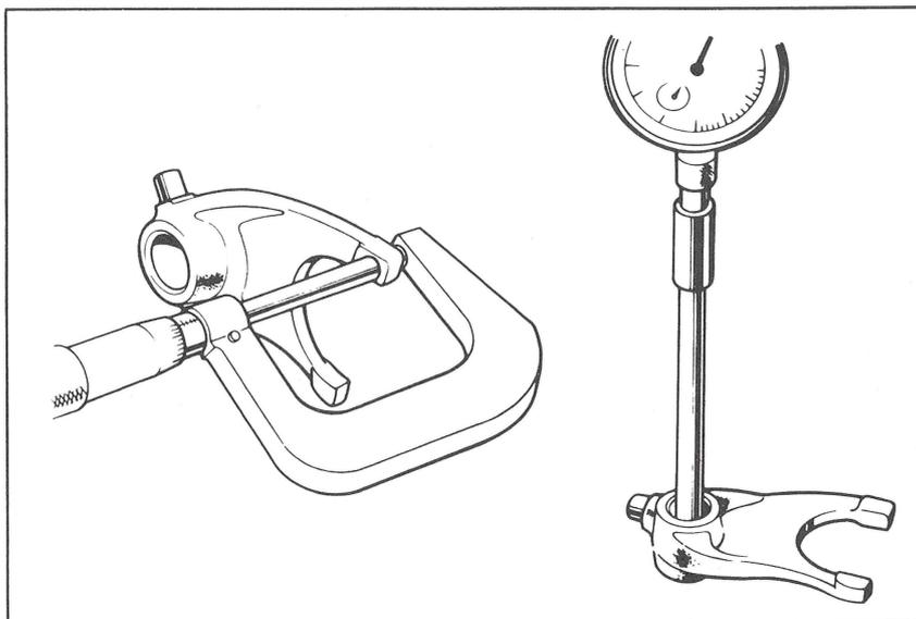
Check the shift fork shaft for wear, damage or bending.
