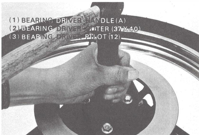
Install the brake disc.
