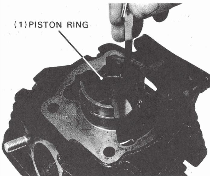
Install the expander in the second groove of the piston. Install the top and second rings (Page 6-7).
