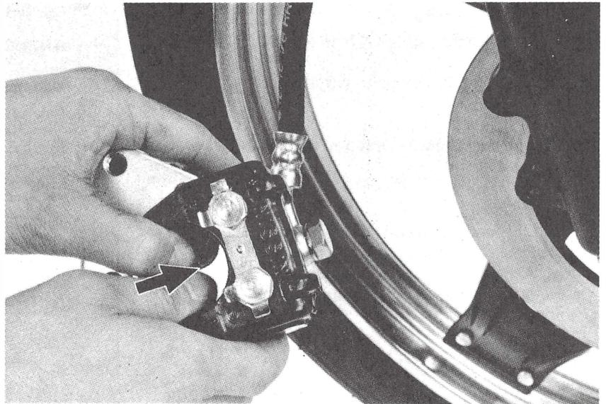
Clean the brake caliper.
