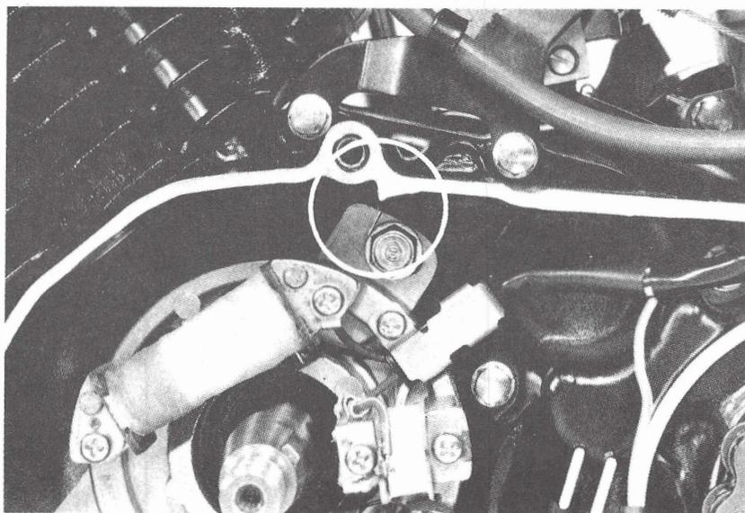
Connect the A. C. generator coupler and neutral switch wires.
