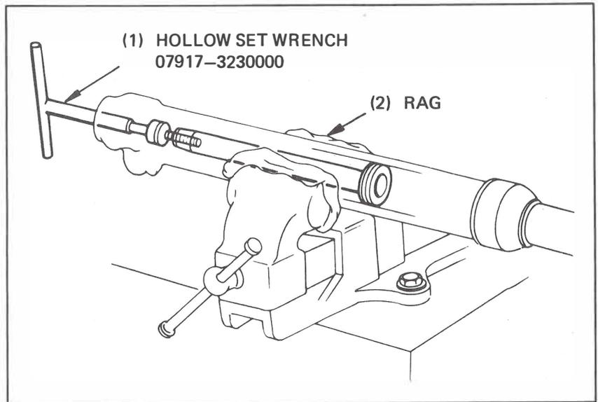
Install the oil seal into the top of the fork slider.
