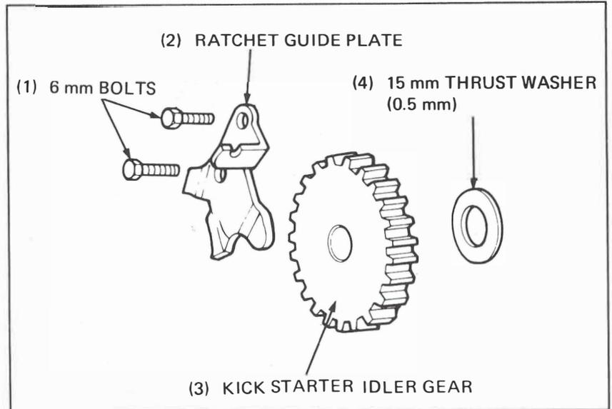
Install the kick starter in the reverse order of disassembly.
