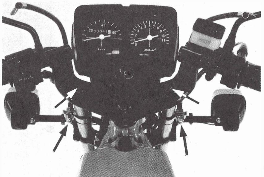
Loosen the fork bottom bridge pinch bolts.
