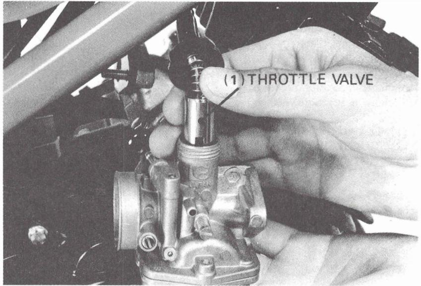
Disconnect the throttle cable from the throttle valve.
