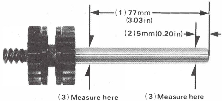
Check the oil pump driven gear for wear or damage.
