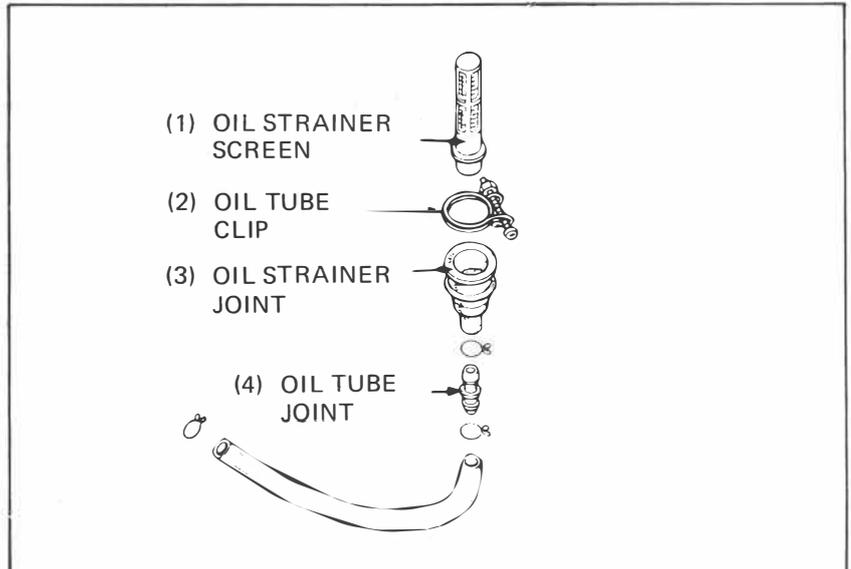
Clean the oil strainer screen with compressed air.
