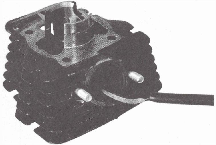
Inspect the cylinder bores for wears at three levels in X and Y directions. Take the minimum figure measured to determine the cylinder wear. Avoid the port area.
