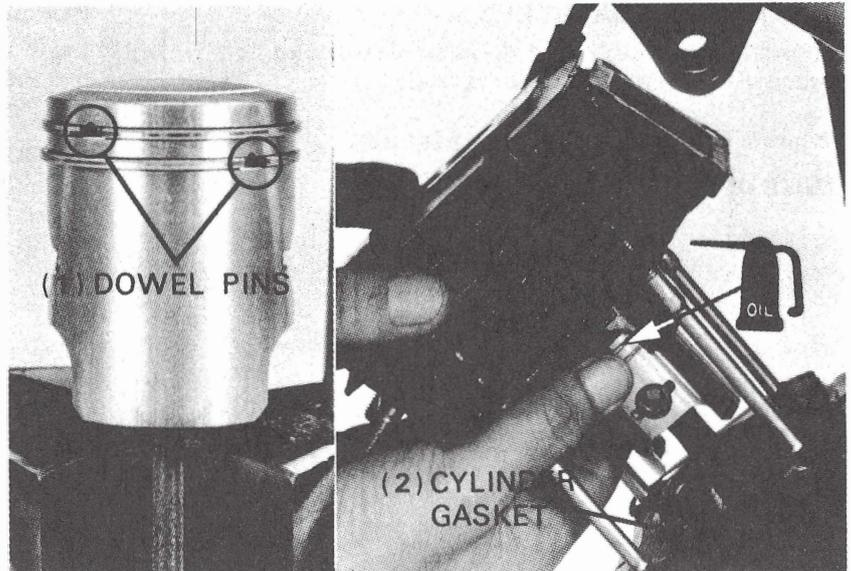
Install the cylinder head on the cylinder with the gasket in between (Page 6-3).
