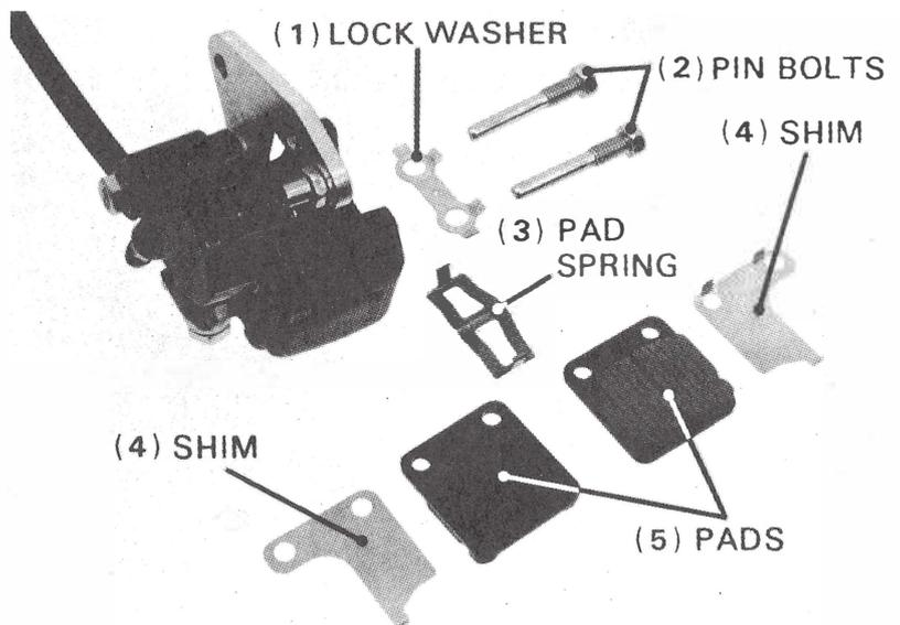
Ensure that the pin bolts are inserted through the holes in the brake pads.
