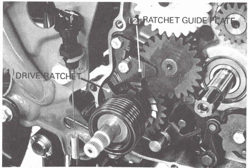
Install the kick return spring. With the balancer properly timed, install the clutch (Page 7-9).
