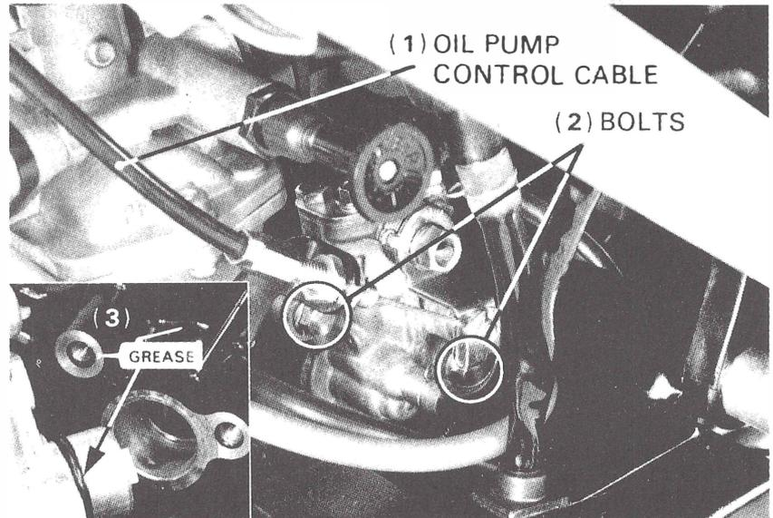
Tighten the oil pump attaching bolts securely.
