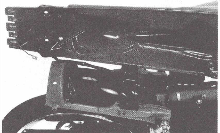
Install the fuel tank mount rubbers as shown.
