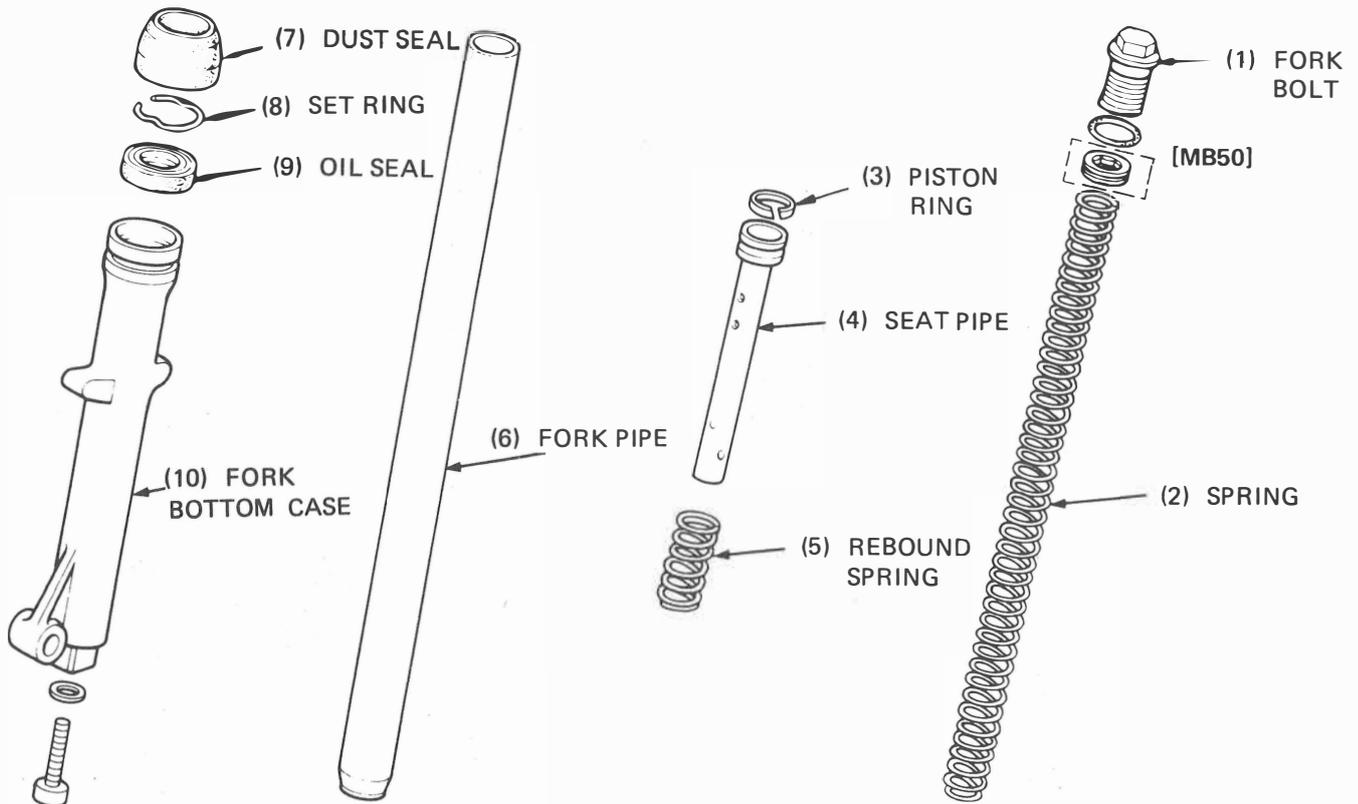
Install the piston ring on the seat pipe.
