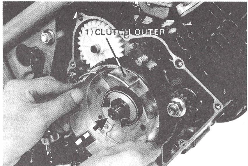
Make sure that the sub gear engages the clutch outer gear properly.
