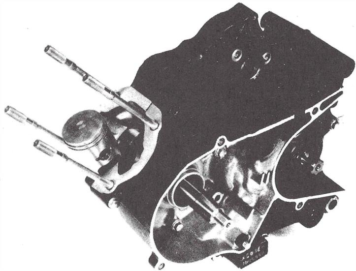
Remove the crankcase attaching bolts.
