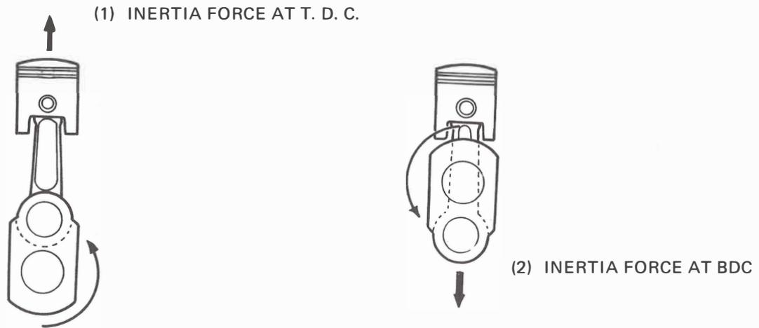
The source of vibration in a reciprocating engine is the "inertia" force created by the rotating or reciprocating masses such as the piston and connecting rod.
