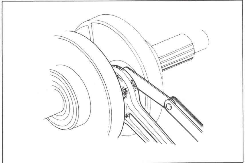
Measure the connecting rod big end radial clearance at two points in the X and Y directions.
