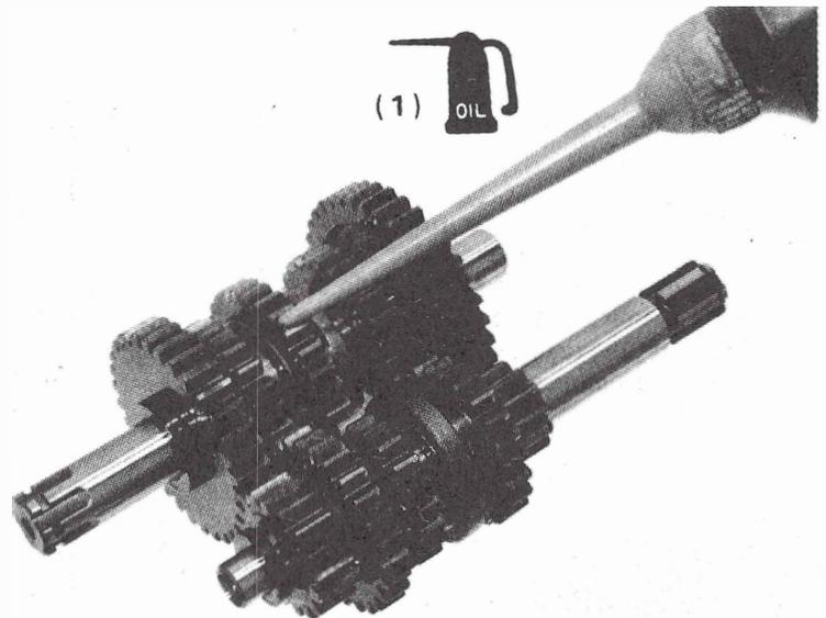
Install the countershaft and mainshaft in the left crankcase.
