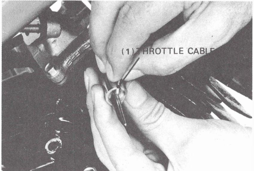
Remove the return spring, carburetor top and sealing cap.
