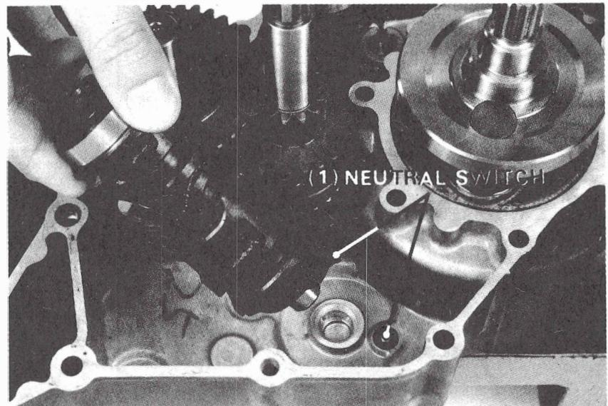
Install the shift drum and shift forks. Slide the shift fork shaft through the shift forks.
