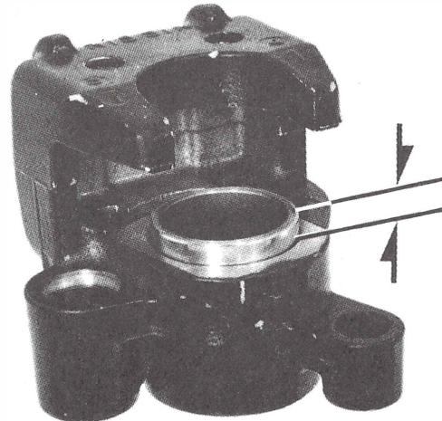
Lubricate the inside of the pin boot with silicon grease and install the bushing in the caliper.
