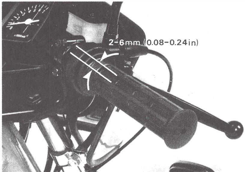
Adjustments are made by loosening the lock nut and turning the throttle grip free play adjuster.
