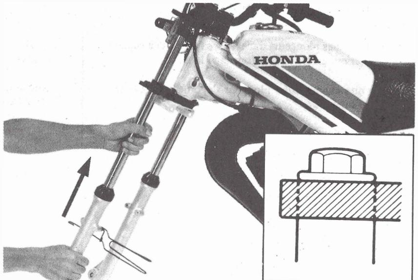
Position the front brake cable guides on the fork top and bottom bridges and install the fork top bridge pinch bolts.
