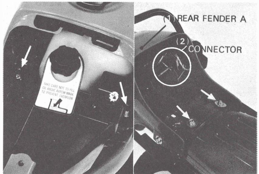
Remove the fuel tank mounting bolts.
