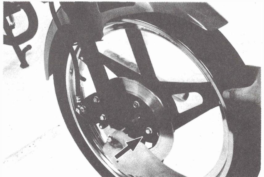
Install a new cotter pin and spread the ends.
