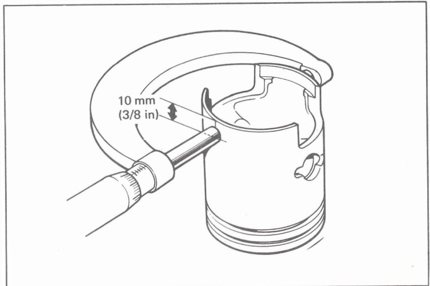
Measure the I. D. of the piston pin bore.
