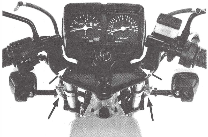
Remove the steering head top thread nut.
