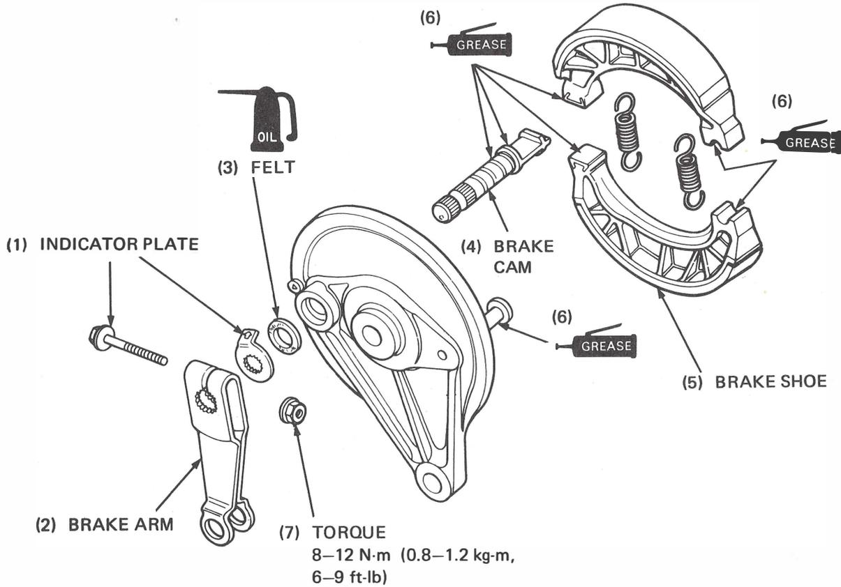
Install the felt ring and wear indicator plate.
