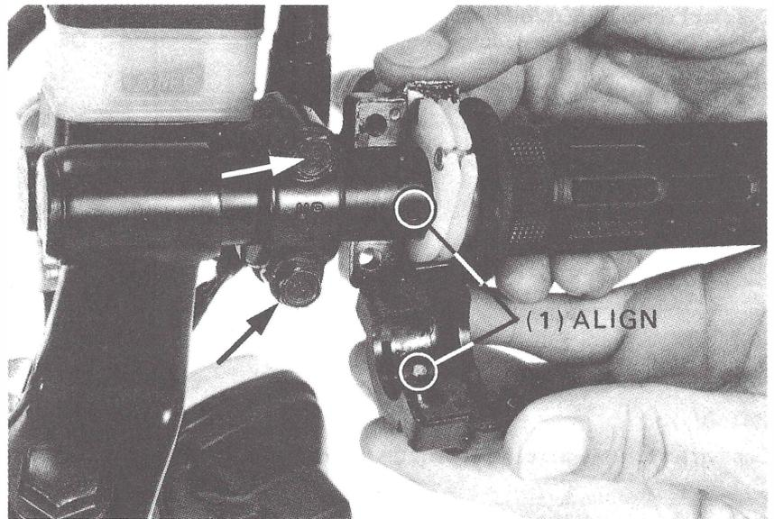
Install the turn signal and dimmer switch assembly with the dowel aligned with the hole in the handlebar.
