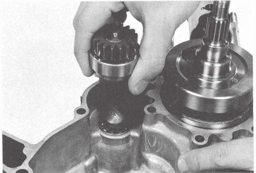
Remove the crankshaft from the left crankcase.
