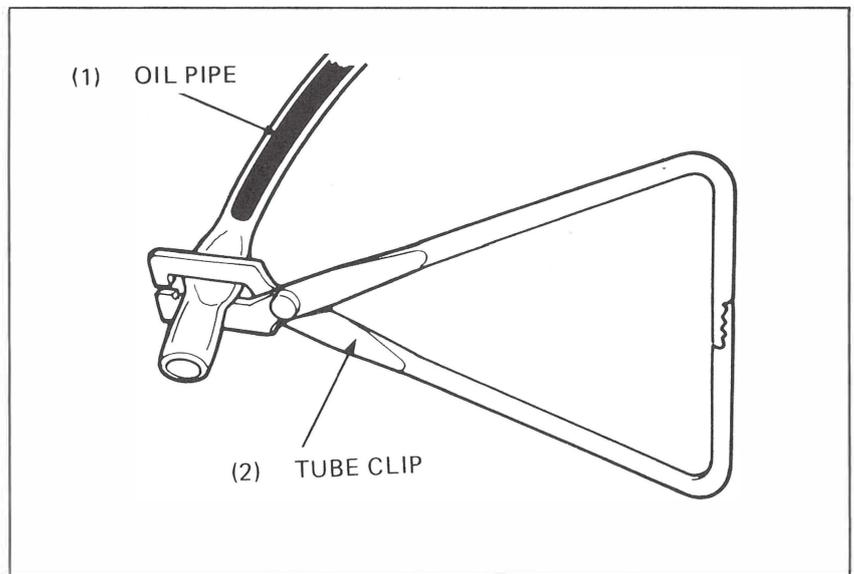
Disconnect the oil pass tube from the inlet pipe.
