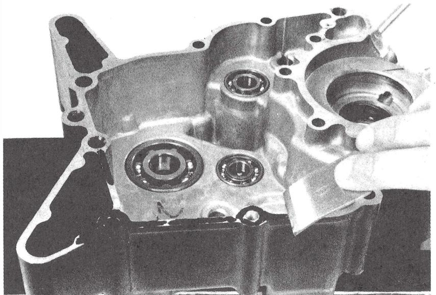
Install the crankshaft in the left crankcase.
