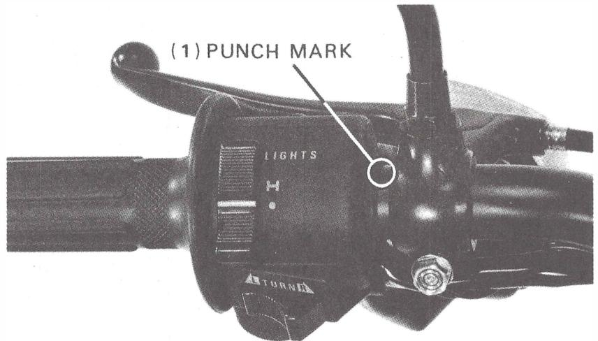
Install the throttle grip and holders on the handlebar aligning the dowel and dowel hole in the holders.
