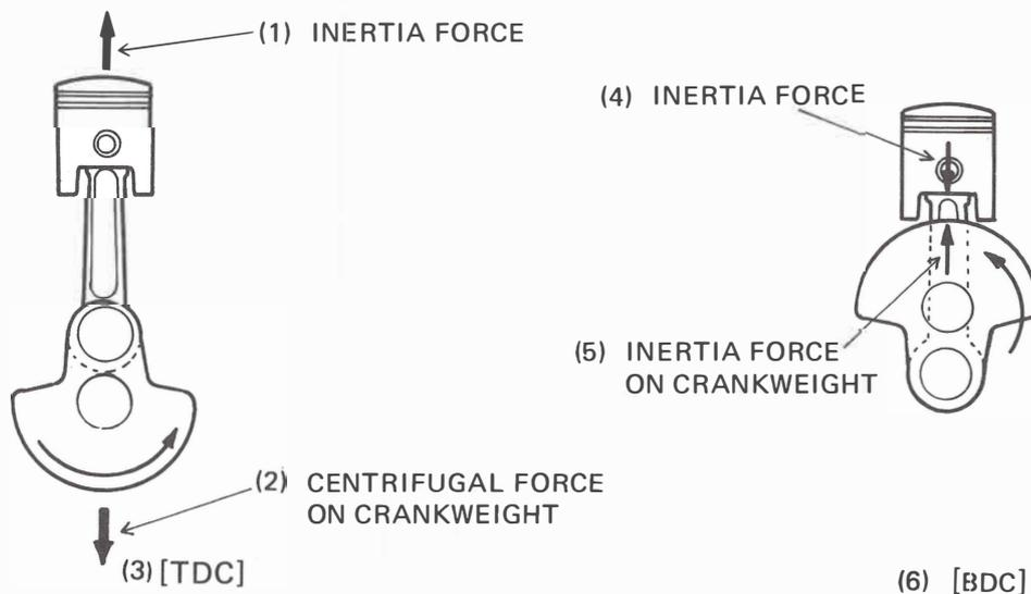
Inertia force created by the rotating mass is in general canceled by counterweights. Their use will reduce vibration caused by the primary inertia force which occurs once every crankshaft revolution. (Hereinafter, inertia force refers to this primary force).
