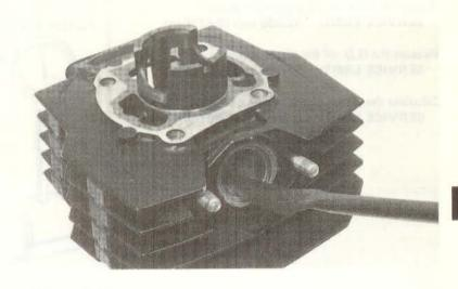
Inspect the cylinder bores for wear at three levels in X and Y directions. Take the minimum figure measured to determine the cylinder wear. Avoid the port area.
