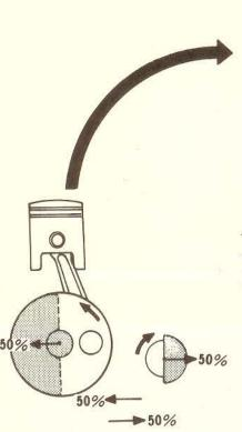
The centrifugal force on the counterweight is balanced by the balancer.
