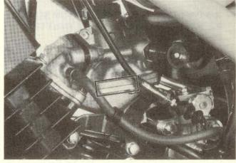
The carburetor identification number is on the carburetor body left side.
