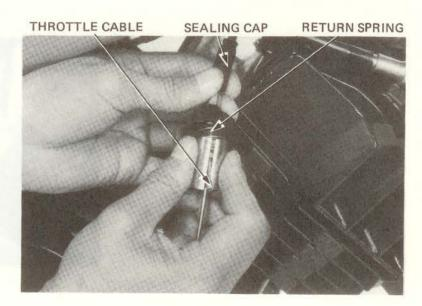
Pry off the cable clip and remove the jet needle.
