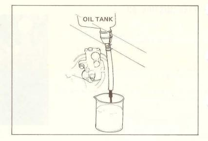
Loosen the tube clip and disconnect the oil tube joint under the oil tank.
