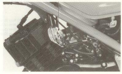
Remove the carburetor flange nuts.
