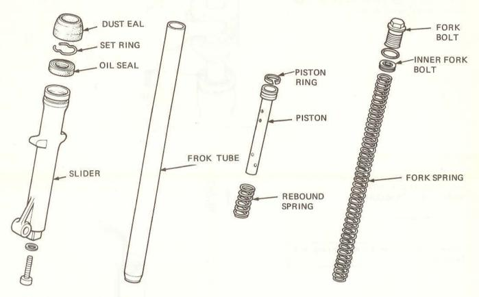
Install the piston ring on the piston.
