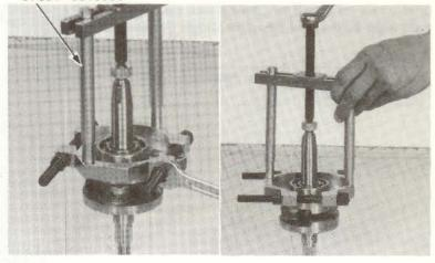
Remove the oil seal and drive out the right bearing from the right crankcase.
