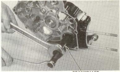
CRANKSHAFT ASSEMBLY TOOL 07965–1660100 BALANCER WEIGHT DRIVER 07945–1660000
