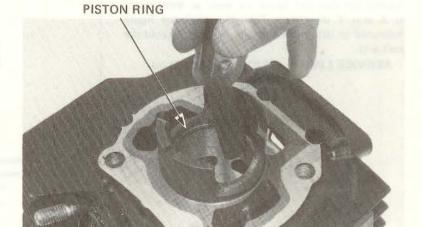
Install the expander in the second groove of the piston. Install the top and second rings (Page 6-7).
