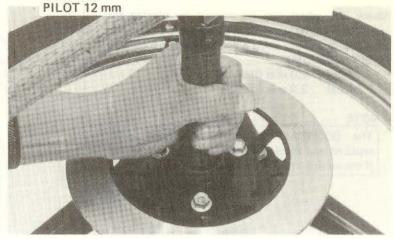
Install the brake disc.
