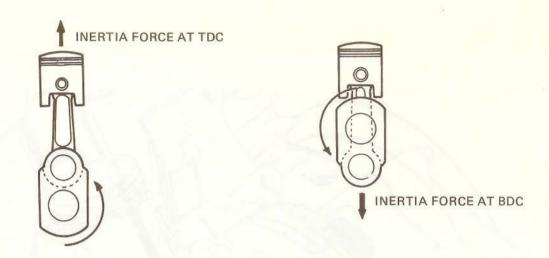
The source of vibration in a reciprocating engine is the "inertia" force created by the rotating or reciprocating masses such as the piston and connecting rod.
