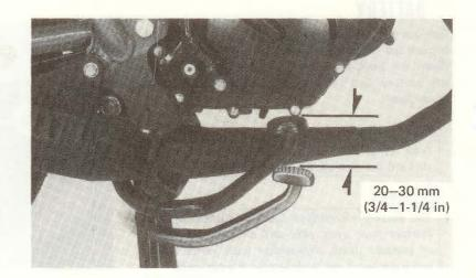
If adjustment is necessary, turn the rear brake adjusting nut.
