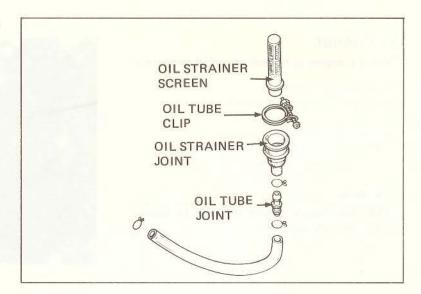
Clean the oil strainer screen with compressed air.
