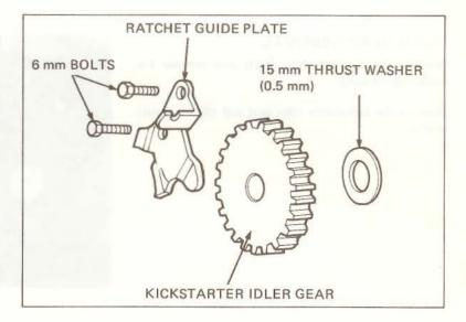
Install the kickstarter in the reverse order of disassembly.
