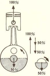
The counterweight creates a centrifugal force to neutralize one-half of the inertia force. The remaining inertia will be totally balanced by the balancer.
