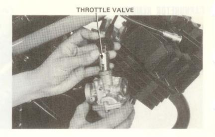
Disconnect the throttle cable from the throttle valve.
