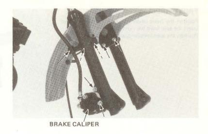
Loosen the fork top and bottom pinch bolts. Remove the front fork.
