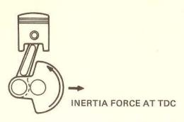
Although the counterweights will balance the inertia force at T.D.C. and B.D.C., they will create a corresponding horizontal imbalance of their own at 90° BTDC and 90° ATDC due to centrifugal force. The balancer is designed to counteract this force including the inertia force created by the reciprocating masses.
