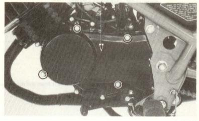
Remove the 12 mm nut attaching the flywheel.
