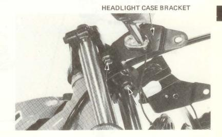
Remove the steering stem nut using a 29 mm socket wrench.
