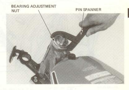
Install the front forks. Install the top bridge. Tighten the stem nut.
