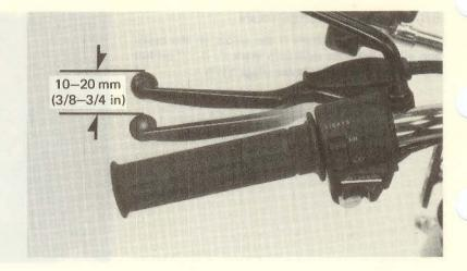
Adjust free play by loosening the lock nut and turning the adjusting nut until the free play is 10–20 mm (3/8–3/4 in).
