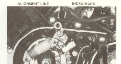
Connect the alternator and neutral switch wires,
