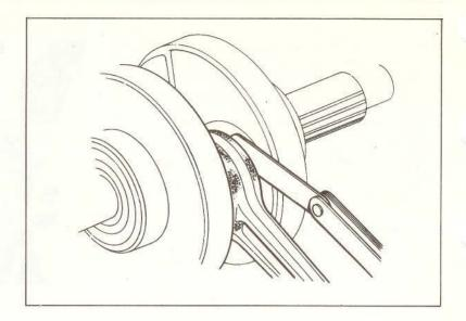
Measure the connecting rod big end radial clearance at two points in the X and Y directions.
