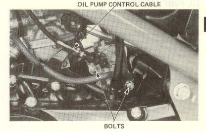
Disconnect the oil pipe from the oil pump, and pinch the end of the oil pipe to prevent oil from flowing out.
