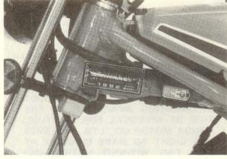
The vehicle identification number (VIN) is near the steering head left side.
