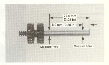
Check the oil pump driven gear for wear or damage.
