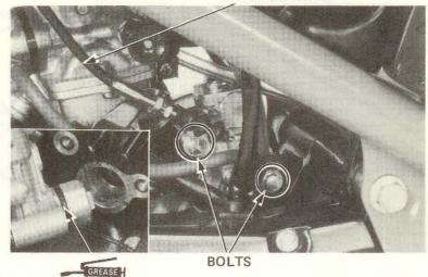
Tighten the oil pump attaching bolts securely. Reconnect the oil pump control cable. Reinstall the oil pipe and oil pass tube.
