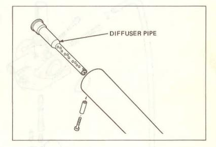
Clean the diffuser pipe with a bristle wire brush. Remove carbon from inside the muffler.
