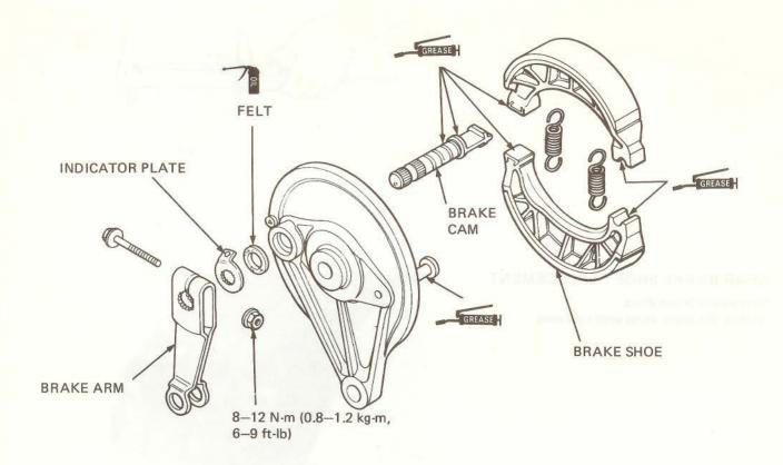
Install the felt ring and wear indicator plate.
