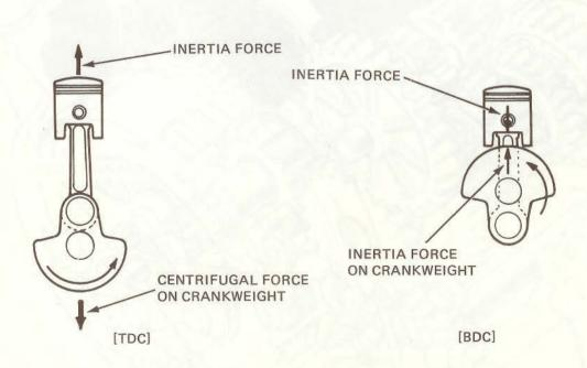
Inertia force created by the rotating mass is in general canceled by counterweights. Their use will reduce vibration caused by the primary inertia force which occurs once every crankshaft revolution. (Hereinafter, inertia force refers to this primary force).
