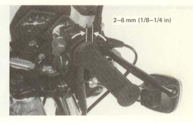
Adjustment can be made at either end of the throttle cable. Minor adjustments are made at the upper end and major adjustments are made at the lower end.
