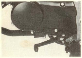
The engine serial number is stamped on the left crankcase.
