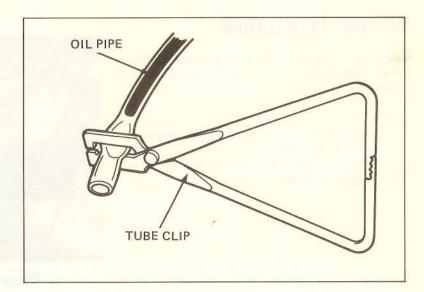
Disconnect the oil pass tube from the inlet pipe.
