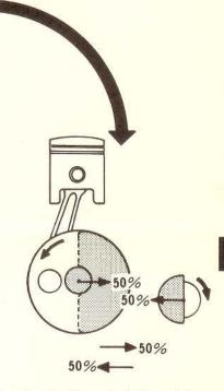
The inertia force is balanced by the counterweight. However, the centrifugal force acting on the counterweight is still present. The centrifugal force on the balancer cancels this remaining force.
