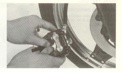
Clean the brake caliper.
