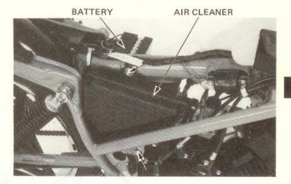
Remove the right and left screws and washers attaching the rear fender B and remove the rear fender B toward the wheel.
