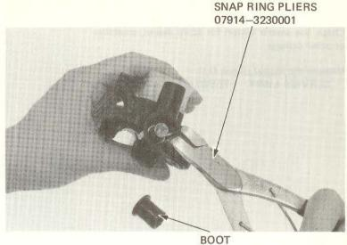
Remove the reservoir from the master cylinder. Clean the master cylinder and reservoir in brake fluid.
