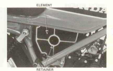
Wash the element in non-flammable or high flash point solvent and allow to dry.
