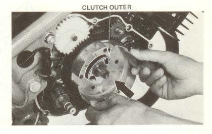
Make sure that the sub gear engages the clutch outer gear properly.
