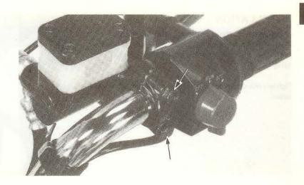
Remove the right handlebar switch and throttle grip.
