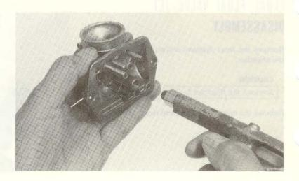
Check each part for wear or damage. Inspect the choke (starter) valve.
