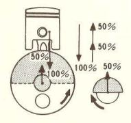
The centrifugal force on the counterweight neutralizes one-half of the downward inertia force. The balancer counteracts the remainder.
