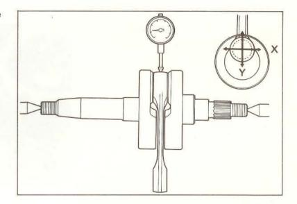
Set the crankshaft on a stand or V-blocks and read runout using a dial gauge.
