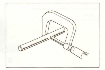
Inspect the shift drum grooves and replace the drum if they are damaged or show excessive wear.
